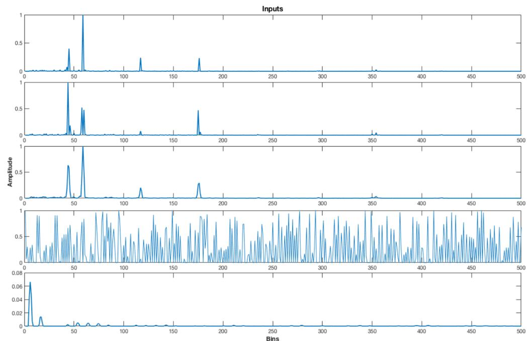
**Figure 8.** System inputs for a chord with 3 pitches (70 + 75 + 94), bottom down—real part of DFT, imaginary part of DFT, radius of DFT, angle of DFT, and real Cepstrum calculated from the time domain signal. Only the first 500 of 2048 bins of all the 5 vectors are shown.
