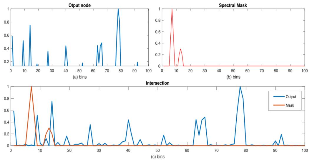
**Figure 10.** (a) CGP output signal, (b) harmonic mask, and (c) computing intersection.
