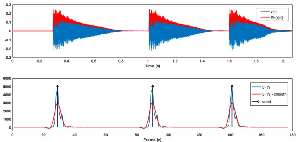
**Figure 3.** Onset detection process—(above) input signal in time domain  $x[n]$  and its Hilbert envelope  $EH[n]$ ; (below) the spectral flux  $SF[n]$ , where  $n$  represents the frame number and the spectral flux smoothed, and in black are the onsets detected and marked.
