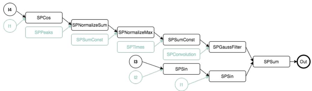
**Figure 16.** Resulting graph after decoding the genotype of classifier 55. The rectangles are functions from the function set, the circles are inputs, and the bold one is the output. In grey are the nodes that are not used to calculate the output due to the arity of some functions.
