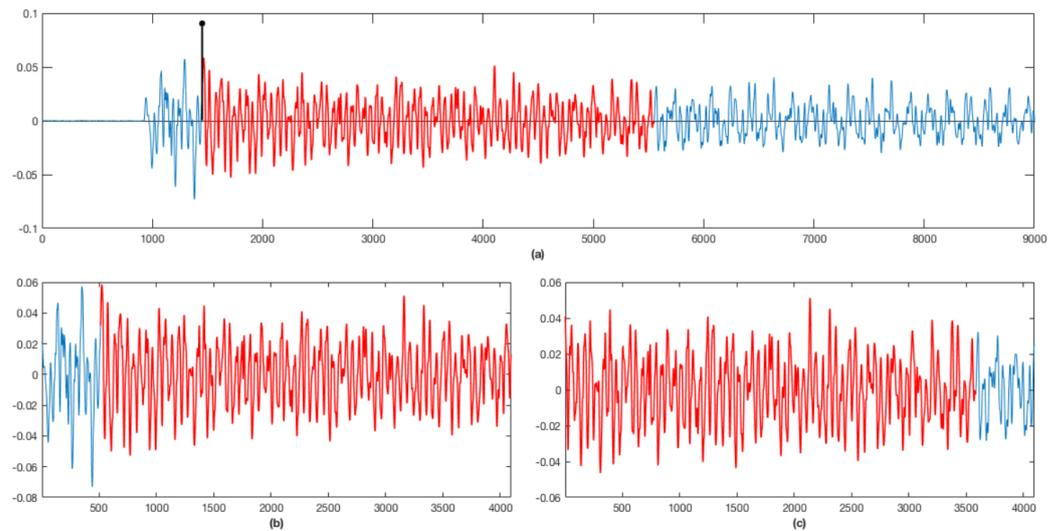
**Figure 6.** Data augmentation process using time translation—(a) in blue is the original piano signal in the time domain ( $\approx 0.2$  s), in black is the inferred onset location  $I_{0s}$ , and in red is the extracted frame, starting at  $I_{0s}$ ; (b) audio frame extracted from the original signal, starting at instant  $I_{0s} - 512$ ; and (c) audio frame extracted from the original signal, starting at  $I_{0s} + 512$ .
