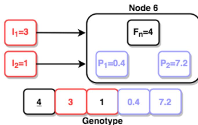
**Figure 9.** Node genotype and its graphical representation. Node 6 has five genes: the first gene (**black**) codifies the function from the function set table (value 4), the second and third genes (**red**) are connection genes (values 3 and 1: node 3 output and node 1 output), and the fourth and fifth genes (**blue**) are real parameters for function use (values 0.4 and 7.2).
