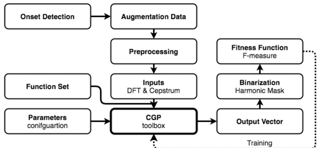
**Figure 5.** Our CGP system block diagram: the training stage starts with a augmentation data process using onset detection, it generates the inputs, the system engine is CGP toolbox that produces the output vector, then binarization and fitness evaluate the individuals and feedback for a CGP toolbox to proceed to the next generation of the evolutionary process.
