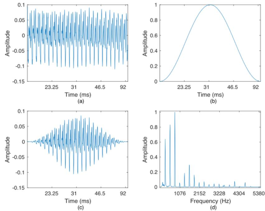
**Figure 7.** Preprocessing—(a) acquired audio frame in the time domain, (b) Hanning window representation, (c) windowed audio frame, and (d) windowed signal represented in the frequency domain after applying the DFT.
