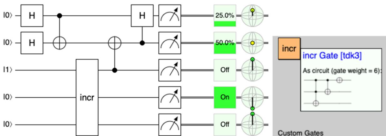
**Figure 9.** Circuit including the reuse of a module (called “incr” and detailed on the right side) with functional cohesion (image obtained using the <https://algassert.com> tool, accessed on 23 June 2021).
