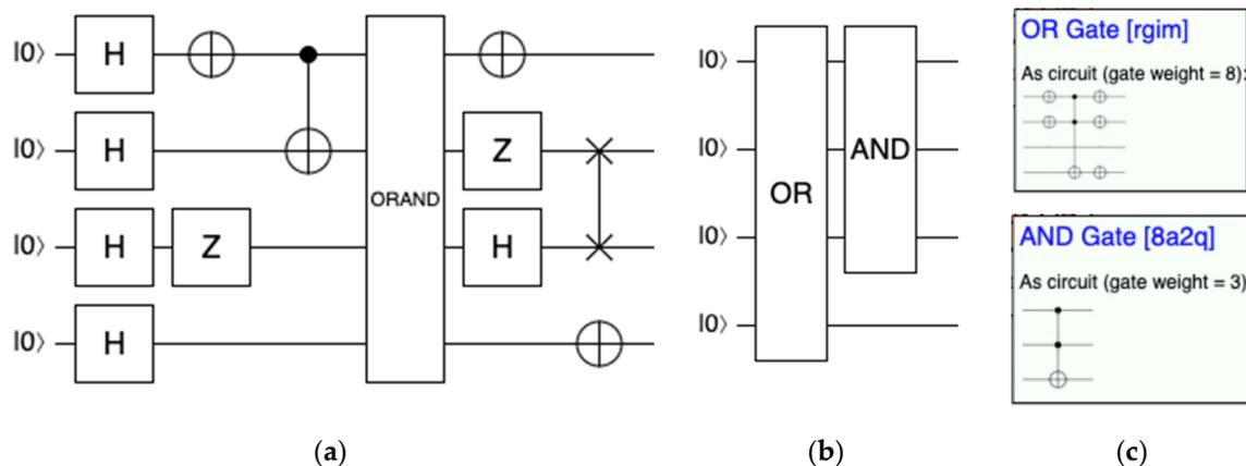
**Figure 10.** (a) A sample of a circuit embedding a module with communicational cohesion. (b) The implementation of the module including OR/AND submodules. The tasks performed within the module (AND/OR operations) share the first three incoming qubits as input data. (c) Detail of the implementation of the submodules.
