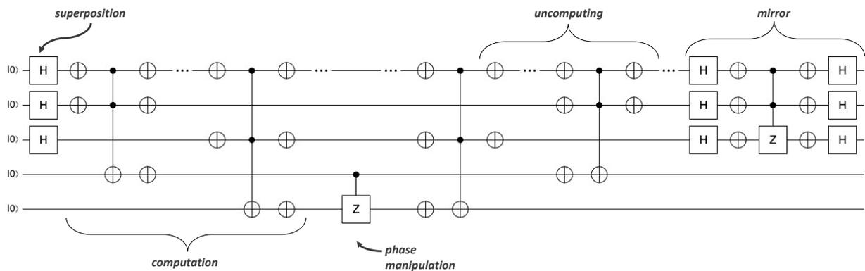
**Figure 8.** Sample of reusable module for solving a 3-SAT to find whether exists a combination of the three Boolean inputs to evaluate as true a given logic expression (image obtained using the <https://algassert.com> tool, accessed on 23 June 2021).
