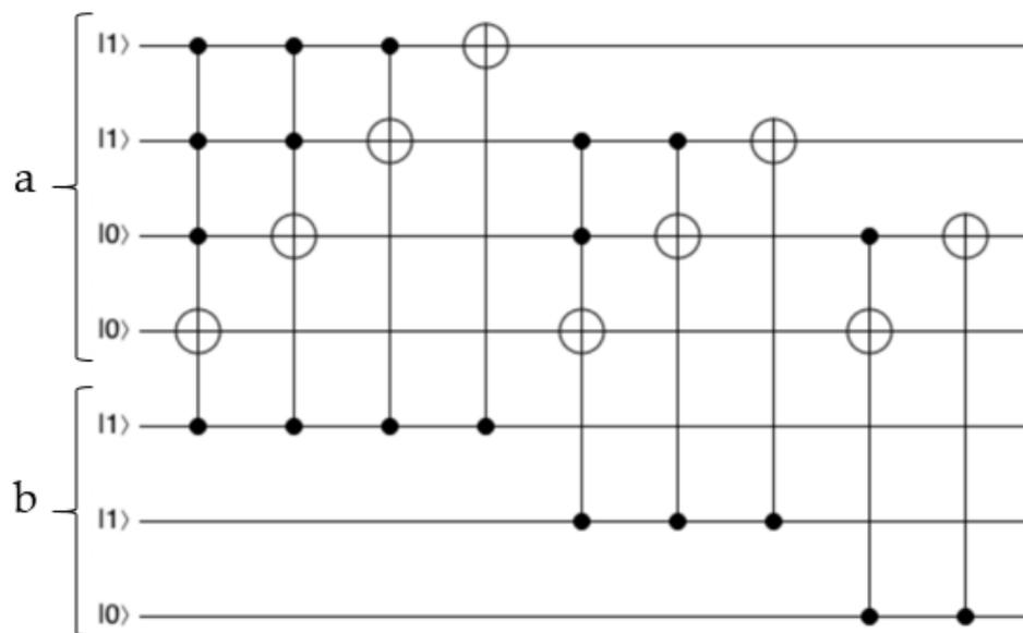
Figure 7. Example of reusable module for adding two numbers represented by the register a and b. Despite it does not include all the elements indicated above, it is a module that fulfils the constraints required to be a module (image obtained using the <https://algassert.com> tool, accessed on 23 June 2021).
