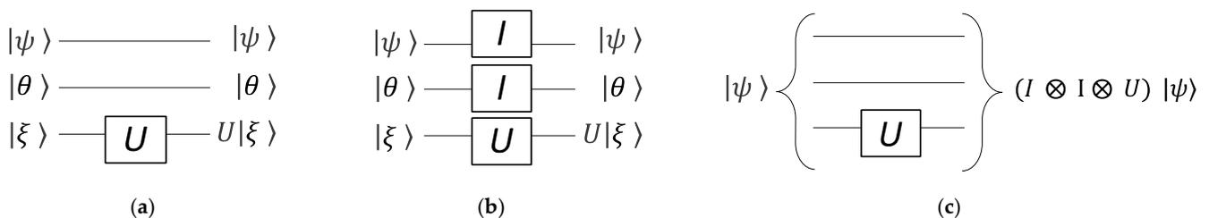
Figure 5. Module with a gate applied to a subset of qubits: (a) a single gate to a qubit; (b) the equivalence using identity gates; and (c) the situation when there is entanglement.
