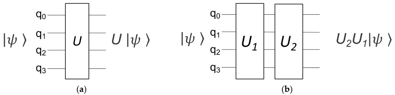
Figure 4. (a) Module a simple gate. (b) Module with two sequential gates.
