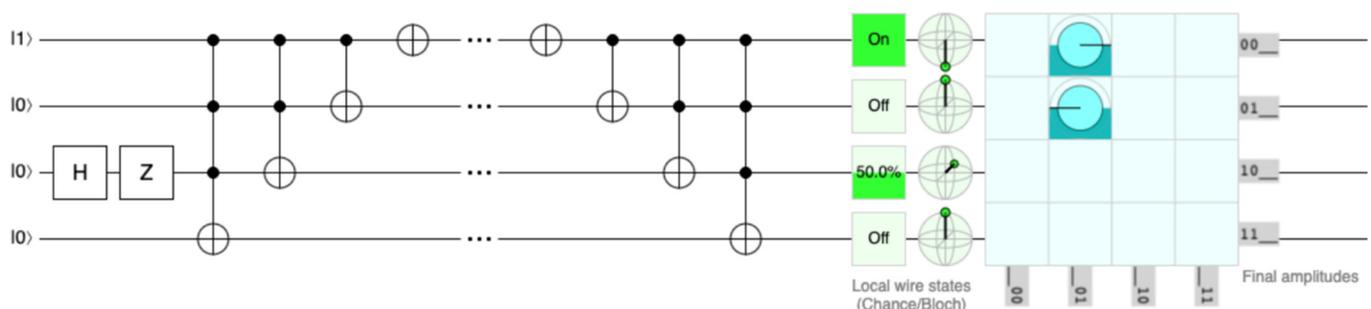
**Figure 2.** A quantum circuit including four qubits and implementing the increment (first part) and decrement (second part) of an integer (image obtained using the <https://algassert.com> tool, accessed on 23 June 2021).
