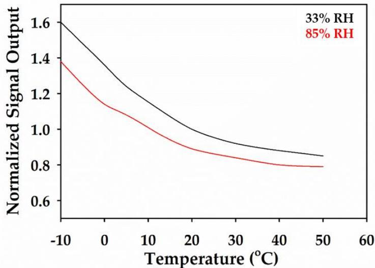
Figure S9. Calibration curve correcting the effects of temperature from -10 to 50 °C at low (33%) and high (85%) relative humidity [2].
