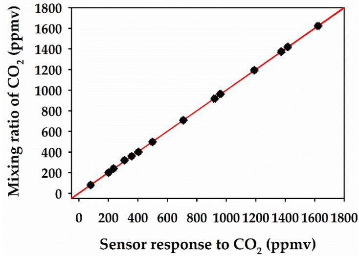
**Figure S2.** Carbon dioxide calibration curve from 80.00-1622 ppmv.  $y = 0.9993x - 1.682$ , where  $y$  represents the concentration of the gas of interest (in parts per billion by volume of air) and  $x$  the response of the sensor. The coefficient of determination for the straight line is  $R^2 = 0.9999$ .
