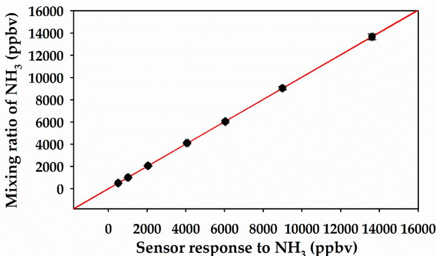
**Figure S3.** Ammonia calibration curve from 500.0-9040 ppbv.  $y = 1.003(x) - 0.0037$ , where  $y$  represents the concentration of the gas of interest (in parts per billion by volume of air) and  $x$  the response of the sensor. The coefficient of determination for the straight line is  $R^2 = 0.9999$ .
