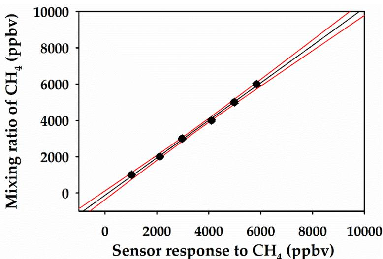
**Figure S1.** Methane calibration curve from 1000-6000 ppbv.  $y = 1.033(x) - 122.0$ , where  $y$  represents the concentration of the gas of interest (in parts per billion by volume of air) and  $x$  the response of the sensor. The coefficient of determination for the straight line is  $R^2 = 0.9981$ .
