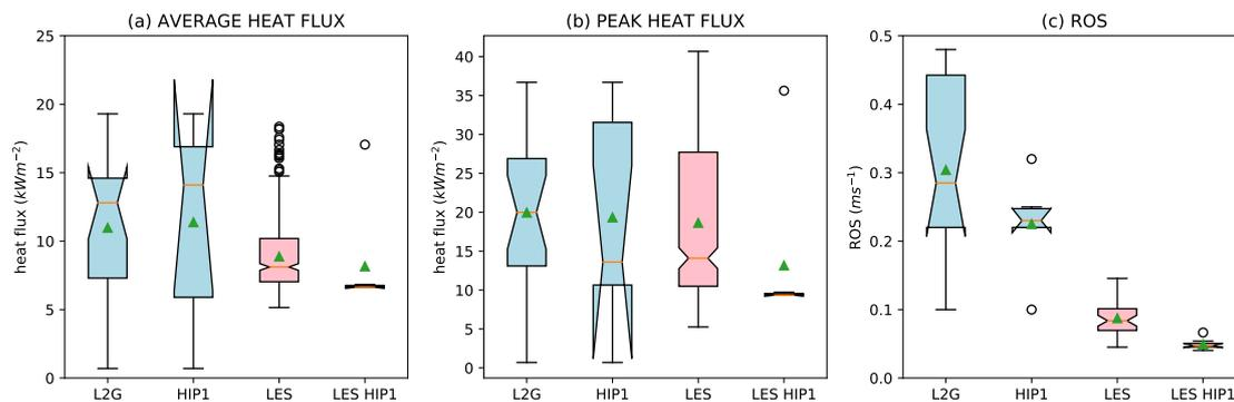
**Figure 3.** Comparison of observed (blue) and modeled (red) fire behavior. The box and whiskers span interquartile range (IQR) and  $1.5 \times \text{IQR}$ , respectively, with the notch denoting the 95% confidence interval of the median ( $\text{median} \pm 1.57 \times \text{IQR}/n^{1/2}$ ). Red line and green triangle correspond to median and mean, respectively. (a) Average heat flux during flaming period. (b) Peak fire heat flux during flaming period. (c) Rate of spread.
