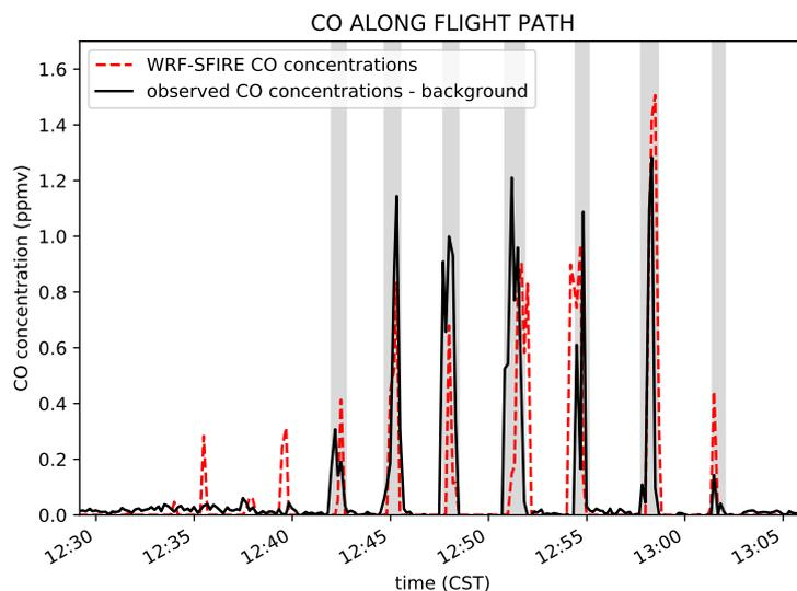
**Figure 4.** Simulated CO mixing ratio along RxCADRE flight path. Red dashed and solid black lines correspond to LES-derived and observed values, respectively. Gray shading indicates observed smoke time periods (not magnitudes) as identified from CO measurements along the flight path.
