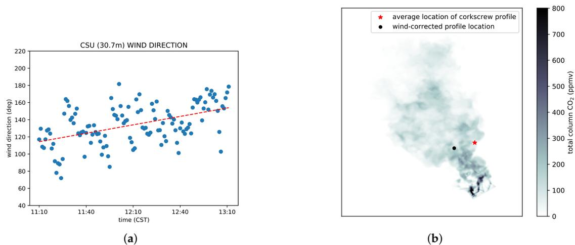
**Figure 6.** The effects of changing mesoscale wind conditions on plume observations (a) Observed change in 30 m wind direction prior to and during the burn. Significant linear trend is shown with a red dashed line. (b) Top view of modeled smoke plume during the “corkscrew” maneuver by the instrumented aircraft. Black dot and red star indicate the average location of the “corkscrew” profile from flight with and without wind-correction, respectively.
