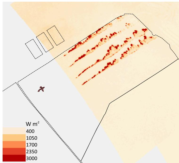
**Figure 1.** Long wave infra-red (LWIR) image of L2G lot during ignition (12:32:02 CST) with dashed black lines denoting burn perimeters. Red scatter points correspond to Highly Instrumented Plot (HIP) #1 fire behavior packages (FBP), each containing a system of airflow, temperature and energy sensors.
