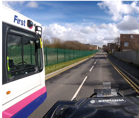
Figure 10. Successful execution of the Bus Trial—Wildcat safely overtaking bus after receiving wireless communication that it is clear to overtake.
