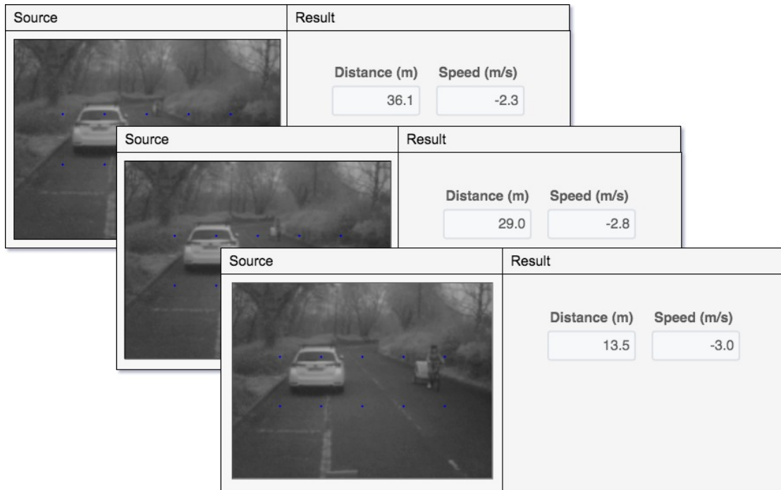
Figure 8. Trial 3 Waiting for oncoming cyclist to pass before overtaking a parked car - scenario viewed through Fusion Processing's sensors.
