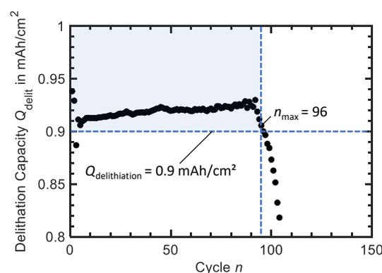
**Figure 3.** Schematic representation of our approach to analyse cycling results. We consider cycling experiments terminated as soon as the delithiation capacity  $Q_{\text{delithiation}}$  of five consecutive cycles drops below  $0.9 \text{ mAh/cm}^2$ . The number of the last cycle with  $Q_{\text{delithiation}} \geq 0.9 \text{ mAh/cm}^2$  represents the maximum number of valid cycles  $n_{\text{max}}$ . Here the cycling performance of an etched brass foil versus Li is shown exemplarily.
