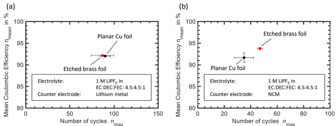
**Figure 4.** Cycle performance of different current collectors for Li electrodes with an electrolyte of 1 M LiPF<sub>6</sub> in EC:DEC:FEC: 4.5:4.5:1 (wt.) represented as the mean Coulombic efficiency  $\eta_{\text{mean}}$  and the mean maximum number of cycles  $n_{\text{max}}$  with standard deviation with  $Q_{\text{lithiation}} = 1 \text{ mAh/cm}^2$  and  $J = 1 \text{ mA/cm}^2$ . (a) Experiments against Li counter electrode (b) Experiments against NCM counter electrode.
