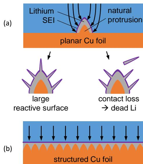
**Figure 1.** (a) Schematic representation of Li deposition on planar Cu foil. Natural protrusions on the surface render inhomogeneous Li deposition. (b) Structured current collectors with large surface area provide numerous nucleation sites and favor uniform deposition.
