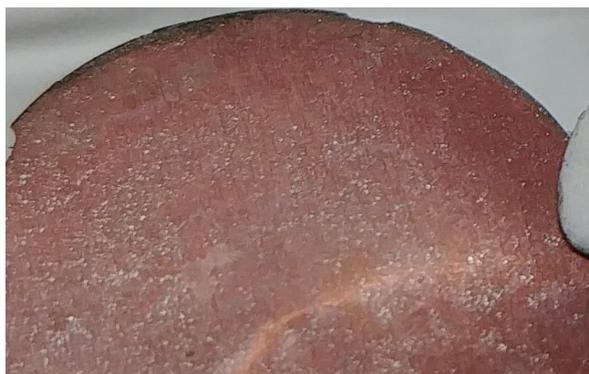
**Figure 6.** Photograph of the backside of a lithiated structured current collector. (The side that was averted from the separator). Li deposits are clearly visible as fine white spots.
