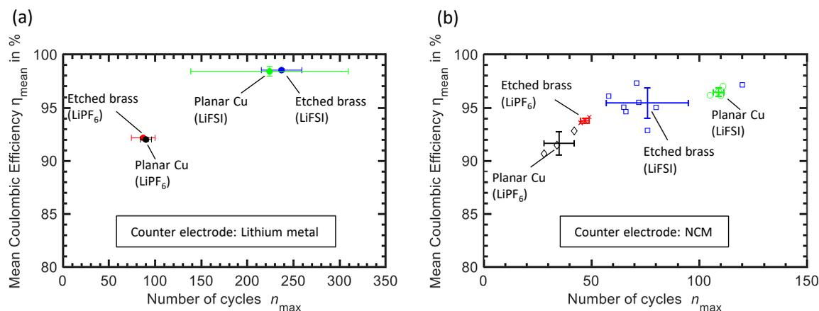
**Figure 7.** Cycle performance of different current collectors with an electrolyte of 1 M LiPF<sub>6</sub> in EC:DEC:FEC: 4.5:4.5:1 (wt.) from Figure 4 and with an electrolyte of 2 M LiFSI in DME represented as the mean Coulombic efficiency and the mean maximum number of cycles with standard deviation. (a) Experiments against Li counter electrode. (b) Experiments against NCM counter electrode. Additionally results of single cells are shown.
