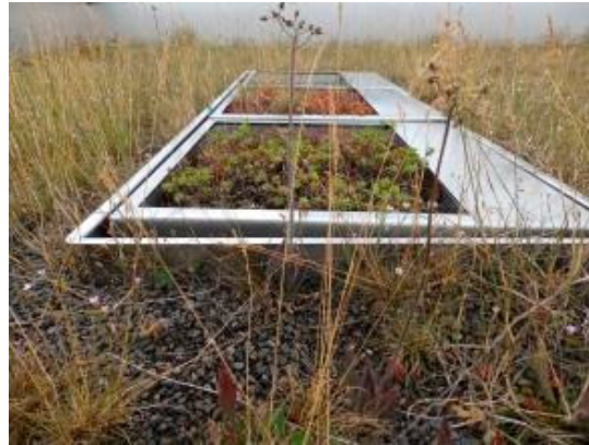
Figure 2. Lysimeter built in an EGR at the University of Applied Sciences in Neubrandenburg, Germany.
