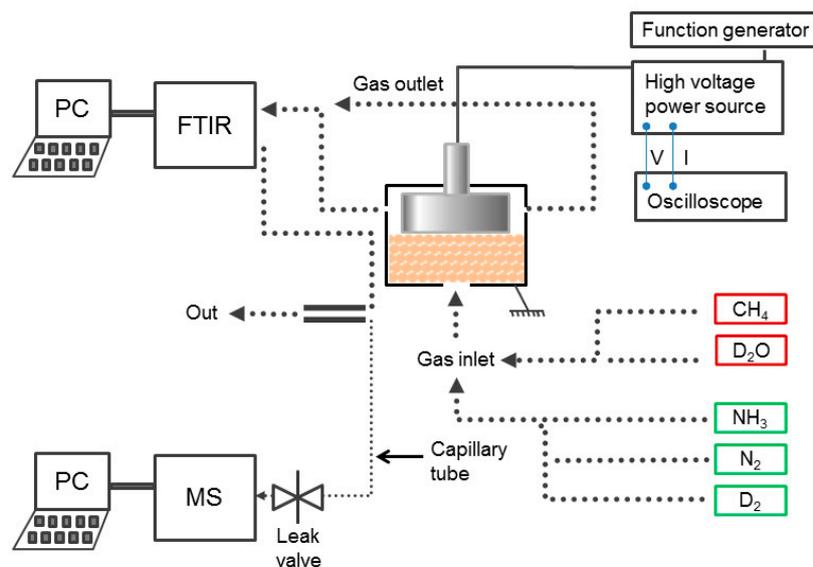
**Figure S4.** Scheme of the experimental set-up. A more detailed description of the reactor and the electrical supply can be found in our previous works [1–3]. Outlet gas flow is represented with the point line.
