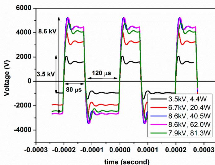
**Figure S5.** Squared AC curves for the different maximum to minimum voltage difference (3.5, 6.7, 8.7, 8.7 and 7.9 kV) and power (4.4, 20.4, 40.5, 62.0 and 81.3 W) in the case of the NH<sub>3</sub>/D<sub>2</sub>/N<sub>2</sub> mixture. Squared signals are expected to provide a higher efficiency than sinusoidal ones due to their higher  $V_{rms}$  value.
