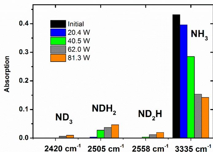
**Figure S3.** Evolution of the intensity of the IR absorption bands attributed to different ammonia species during isotope labelling processes induced by DBD plasma.
