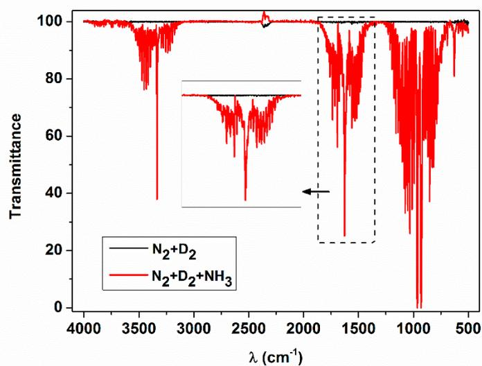
**Figure S2.** FTIR spectra recorded for binary  $N_2+D_2$  (black line) and ternary  $N_2+D_2+NH_3$  (red line) mixtures before plasma ignition. This analysis disregards the presence of water in the reactor chamber, since the zone  $1300-2000\text{ cm}^{-1}$  only presents bands for the ternary mixture, which correspond to  $NH_3$ .
