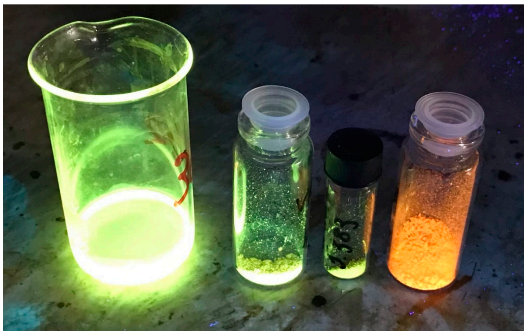
Figure 4. Fluorescence of compounds 4a (solution in \text{CHCl}_3 ), 4a (solid), 4a' and 4h under 365 nm light. Differences in brightness between isomers 4a and 4a' can be seen.
