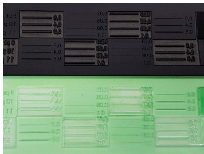
Figure 20. Line elements on EPDM plate (black) and photopolymer plate (green).
