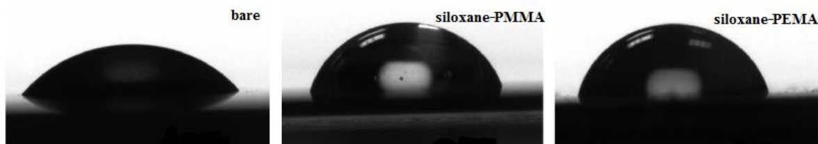
Figure S1. Images of water drop on bare substrate AA7075-T6 and coatings siloxane-PMMA and -PEMA.
