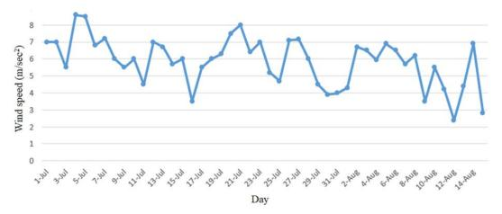
**Figure 13.** Measured wind speed at the site under study (Assiut University, Egypt) at the maximum solar radiation per day.
