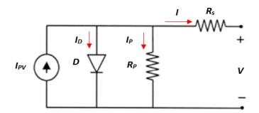
Figure 5. Equivalent circuit of the single diode model (SDM).
