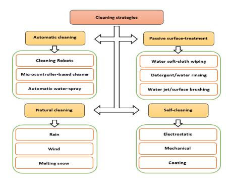
Figure 2. Different cleaning strategies for removing dust from solar PV panels.
