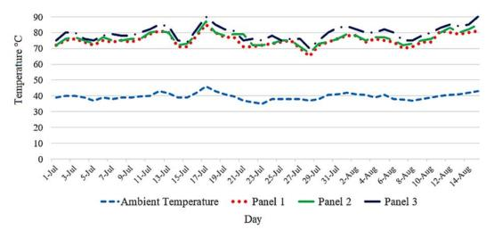
**Figure 14.** Average daily temperature; ambient and the three panels' temperatures at the maximum solar radiation per day.
