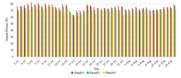
**Figure 11.** The average power generated by the three panels (during 2019); panel 1: SiO<sub>2</sub> nano-coated panel; panel 2: manual cleaning panel without a coating of any material; panel 3: dusty panel.
