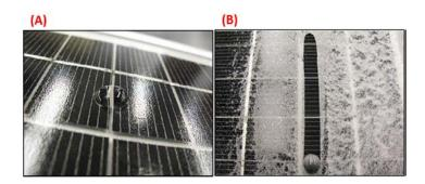
**Figure 3.** Self-cleaning hydrophobic coatings; (**A**) nanomaterial coated solar PV panel, and (**B**) water rolls off the surface like a sphere rolling down a slide.
