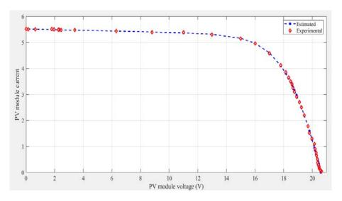
**Figure 15.** Comparison between the experimental and estimated *I-V* data of PV panel which was coated with SiO<sub>2</sub> nanomaterial.
