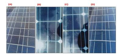
Figure 7. Process of surface self-cleaning with nano-coated material; starting from (A) dirty panel throughout (B) partially cleaned panel, then (C) almost cleaned panel, and finally (D) totally cleaned panel.
