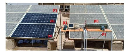
**Figure 6.** Picture of experimental set-up during measuring work. (**A**) Self-cleaning panel coated with  $SiO_2$  hydrophobic nanomaterial, (**B**) uncoated panel—manual cleaning, (**C**) dusty panel, over all the time of the experiment (reference), (**D**) load (variable resistance) and (**E**) measuring devices.
