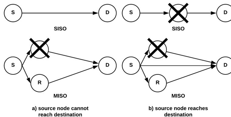
**Figure 4.** Single-in-single-out vs. Multi-in-single-out (CC) with a corrupt relay node.
