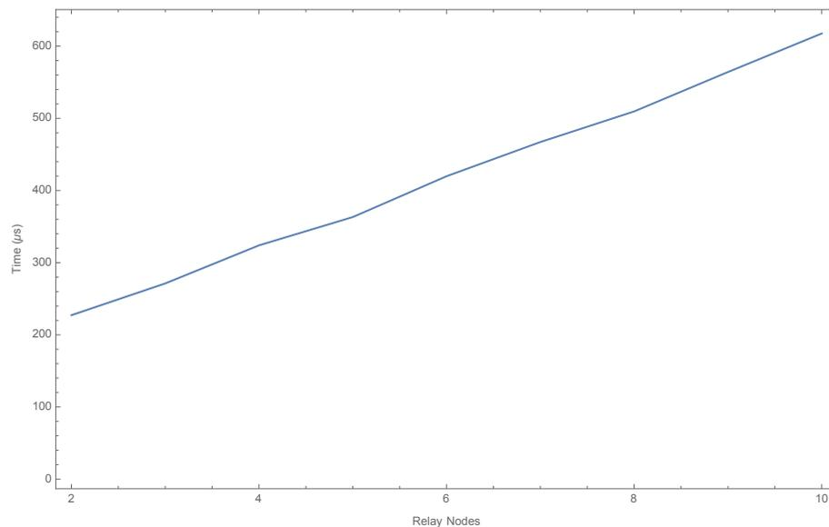
**Figure 5.** Linear relationship between number of nodes and total average time of execution with 1 input byte.
