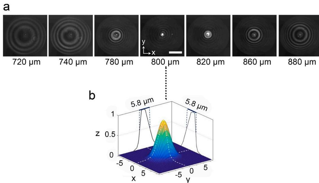
**Figure 4.** (a) The measurement of the intensity distribution at different locations from the metasurface for 1064 nm laser light with 30 mW power. The scale bar is 50 μm. The laser beam was focused sharply at 800 μm corresponding to the design. (b) The interpolated surface plot from the intensity measurement at 800 μm gives a full width at half maximum (FWHM) spot size of 5.8 μm.
