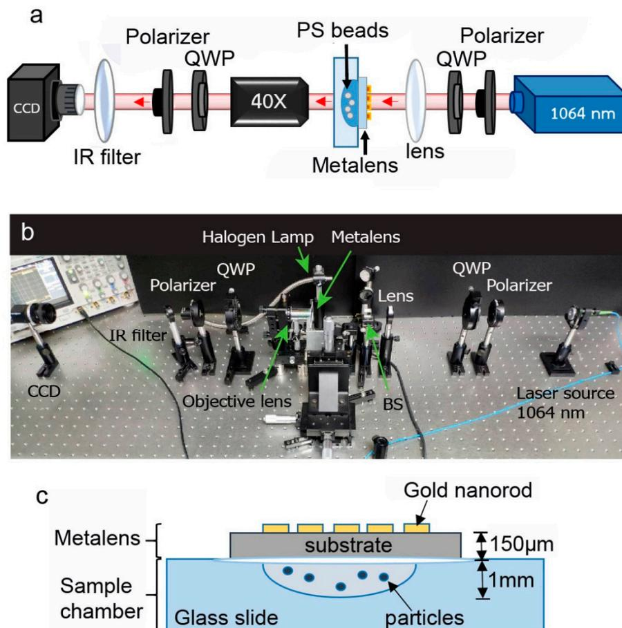
**Figure 3.** (a) An experimental setup diagram of metalens based on optical tweezers with (b) a laboratory setup illustrated. Note that a straight beam path from the laser to a CCD camera is for optical trapping and an illumination path with a halogen lamp as a light source is set on the side to enter the optical trapping path through a beamsplitter (BS). (c) Schematic sketch of the chambered glass slide, which was attached on top with metalens as a sample container.
