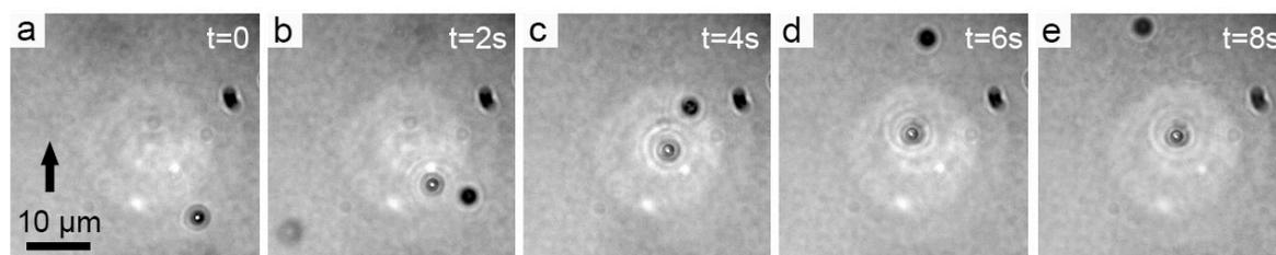
**Figure 6.** A video sequence recorded during trapping of a PS bead: (a,b) bead flowed up due to heat convection of laser spot (c) bead entered into the trap and (d,e) remained in the trap while others on the background kept flowing up. Arrow indicates the bead of interest flowing in an upward direction.
