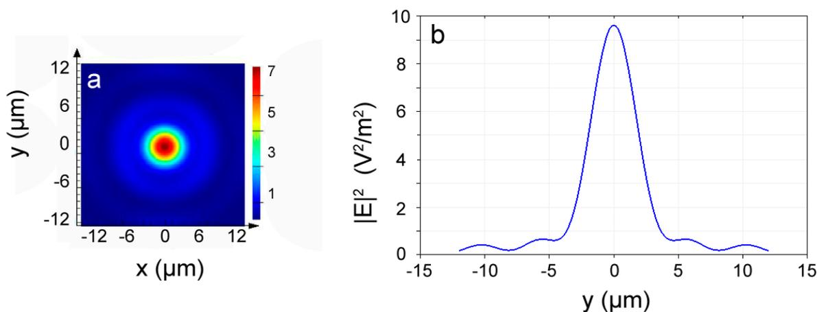
**Figure 5.** (a) The calculated intensity profile of the focal spot of the metasurface calculated by Lumerical FDTD simulation and (b) its vertical cut of the beam through x-z plane with an FWHM of 5.4 μm.
