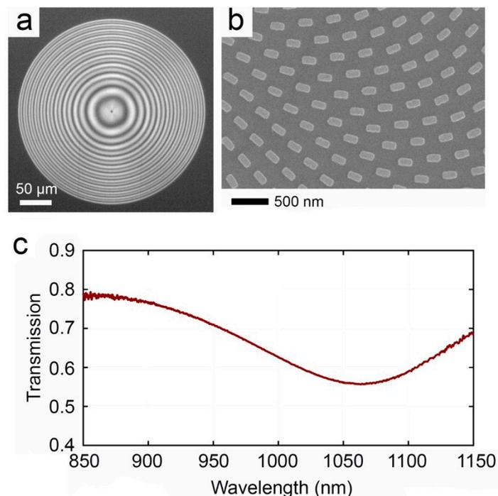
**Figure 2.** The schematic of plasmonic metalens designed for the focal length of 800  $\mu\text{m}$ . (a) Optical microscopy image of the metalens surface. The scale bar is 50  $\mu\text{m}$ , (b) SEM image of part of the lens showing the gold nanorods. The scale bar is 500 nm. (c) Measurement of the FTIR transmission spectra of the metalens showing localized surface plasmon polariton resonance at 1064 nm.
