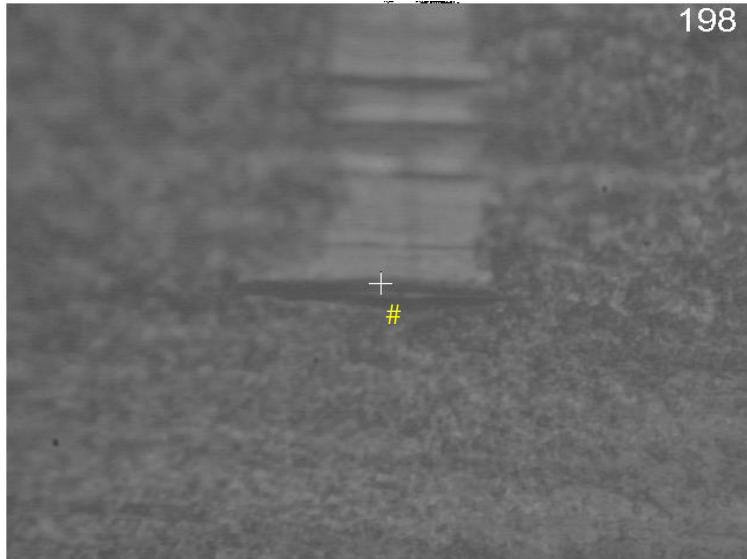
Figure S7. The microhardness indentation of caries lesion bovine dental enamel treated with Neutraçucar. This microscopic image was captured in a microhardness program (40×). # indentation
