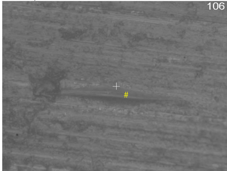
Figure S5. The microhardness indentation of caries lesion bovine dental enamel treated with Colgate 12. This microscopic image was captured in a microhardness program (20 \times ). # indentation
