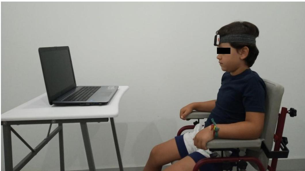
**Figure 1.** Inertial measurement unit (IMU) test application: sensor, subject, and laptop location.
