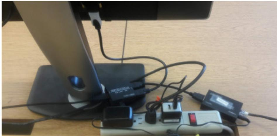
**Figure 7.** Components of a student station. Shown are a  $1 \times 2$  HDMI splitter and HDMI over CAT5 transmitter.
