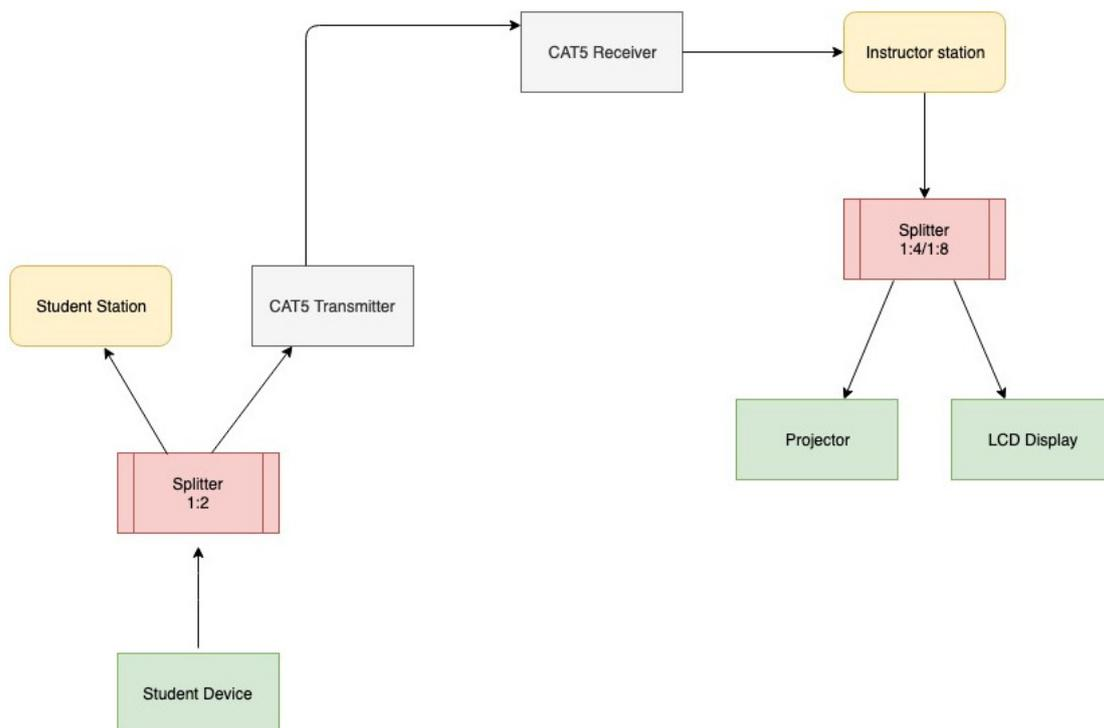
Figure 6. An example architecture of a featherweight hardware-based system for collaboration. Student stations use  $1 \times 2$  splitters to simultaneously mirror content locally and send to an instructor station. At the instructor station, a switch is used to select between inputs and an additional splitter is used to route the selected signal to an instructor display/projector and larger LCDs.
