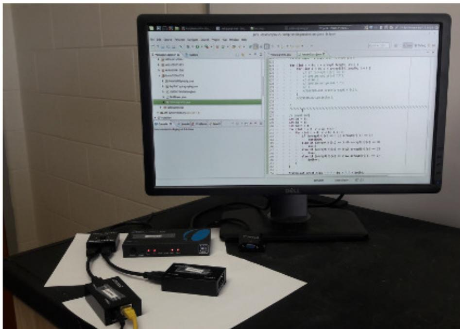
**Figure 8.** Components of an instructor station. Shown are two HDMI over CAT5 receivers, an HDMI switch and a  $1 \times 4$  HDMI splitter with one output connected to an instructor display. The additional outputs from the HDMI splitter could be sent to larger LCDs placed around the classroom.
