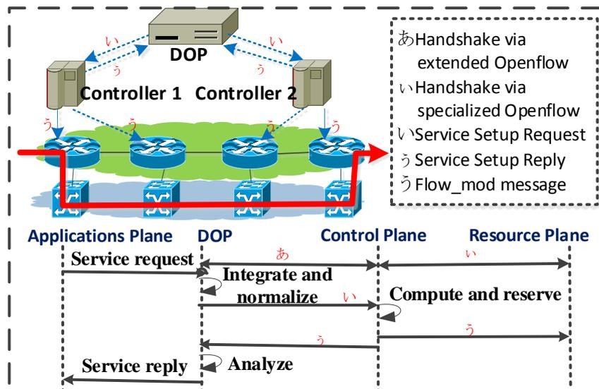
**Figure 2.** The demonstration for signal process of unified multi-layer (UML).
