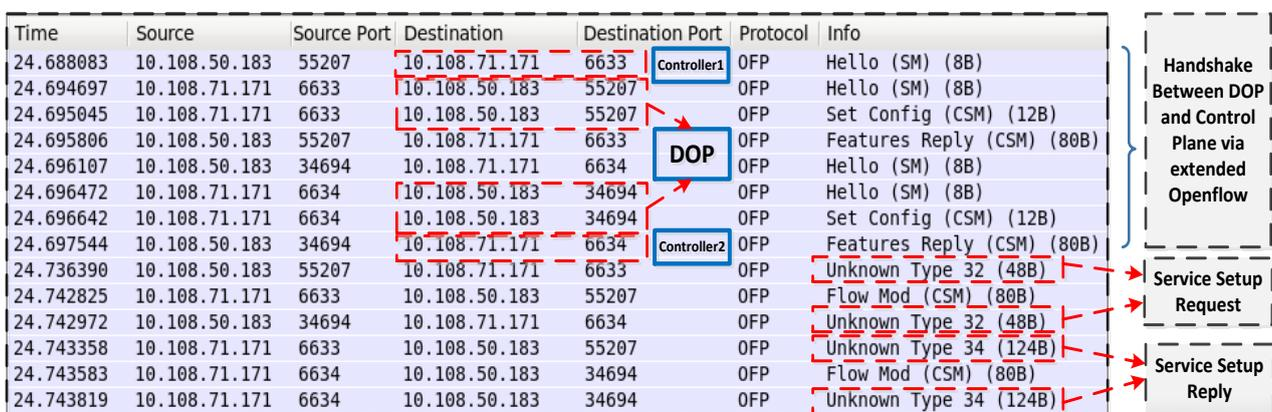
Figure 3. Wireshark capture of the signal processing for the UML architecture.
