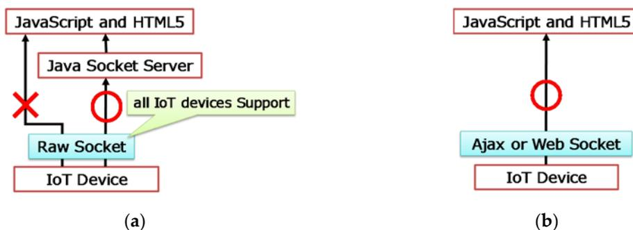
Figure 14. Communication with IoT device. (a) IoT device only supporting raw socket; (b) IoT with Ajax or WebSocket.
