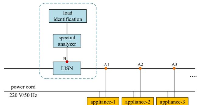
Figure 3. Schematic diagram of the measurement system. LISN, line impedance stabilization network.
