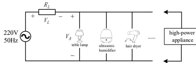
Figure 6. Schematic diagram of the power grid.
