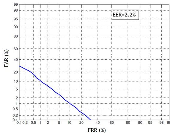
**Figure 5.** Detection of Error Trade-off (DET) plot showing an Equal Error Rate (EER) of 2.2%. FFR, False Fake Rate; FLR, False Living Rate.
