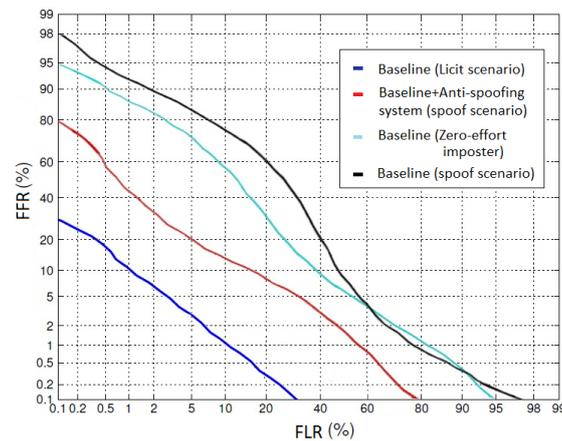
**Figure 6.** False Fake Rate (FFR) and False Living Rate (FLR) of the proposed biometric system with/without spoof-attack.
