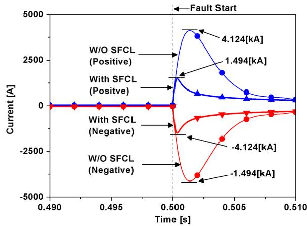
Figure 4. Fault Current according to apply or not SFCL.
