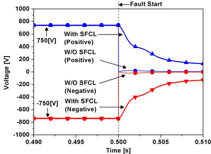
Figure 5. DC Voltage in LVDC system according to apply or not SFCL.
