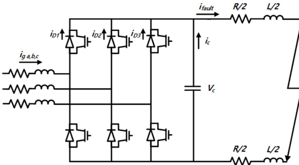
Figure 3. Equivalent Circuit for Short Circuit Fault in LVDC System.
