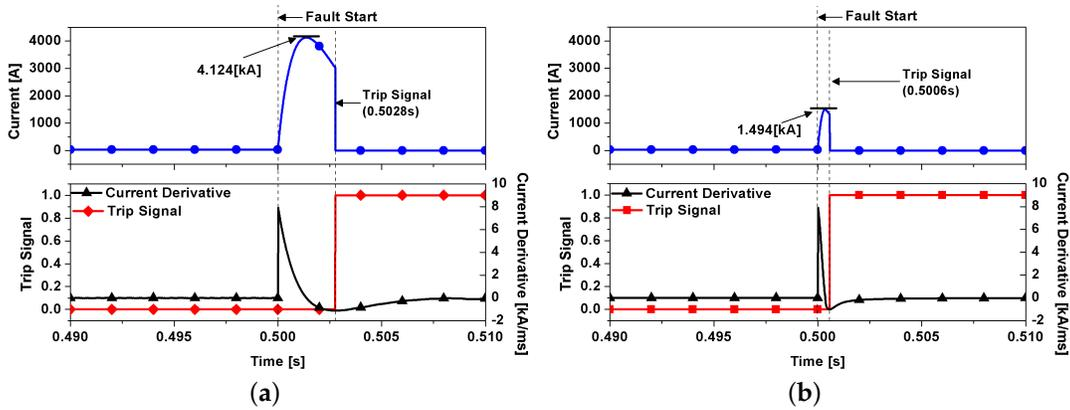
Figure 8. Fault Current and Trip Signal in Selective Protection Relay (a) W/O SFCL (b) With SFCL.
