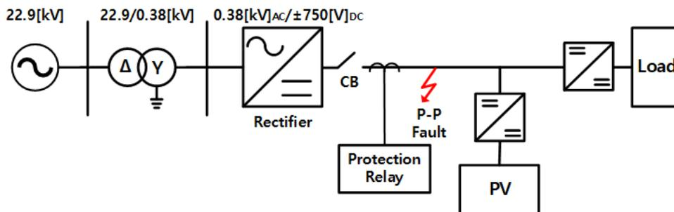
Figure 1. Modelling of low voltage direct current (LVDC) System.
