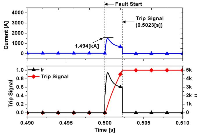
Figure 7. Fault Current and Trip Signal when using the voltage component of high temperature superconductivity (HTSC) element.
