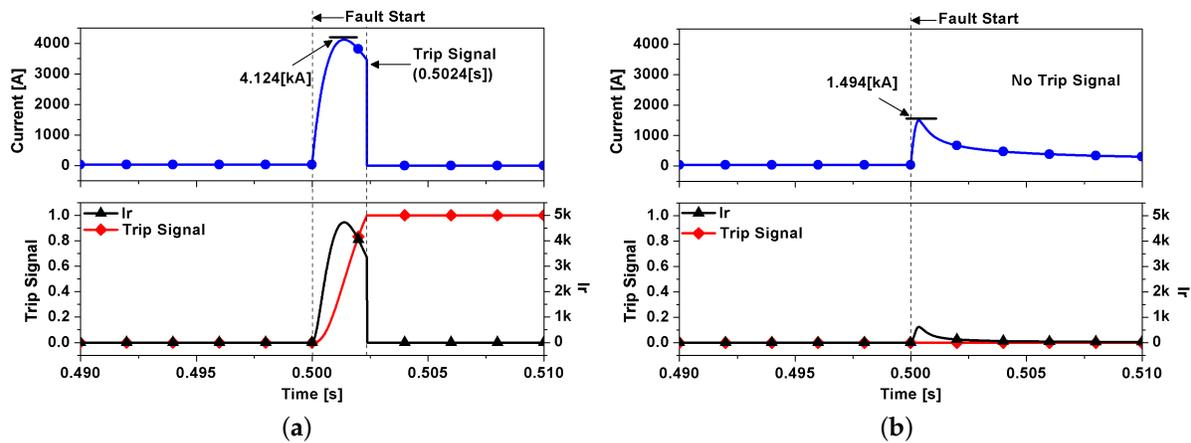
Figure 6. Fault Current and Trip Signal in Over Current Relay (a) W/O SFCL (b) With SFCL.
