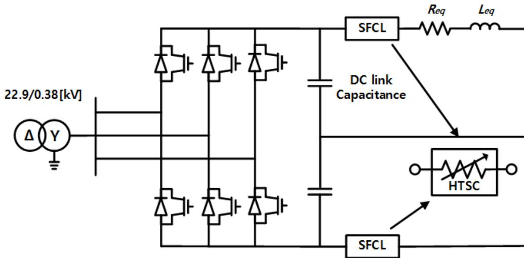
Figure 2. Concept of SFCL on LVDC system.
