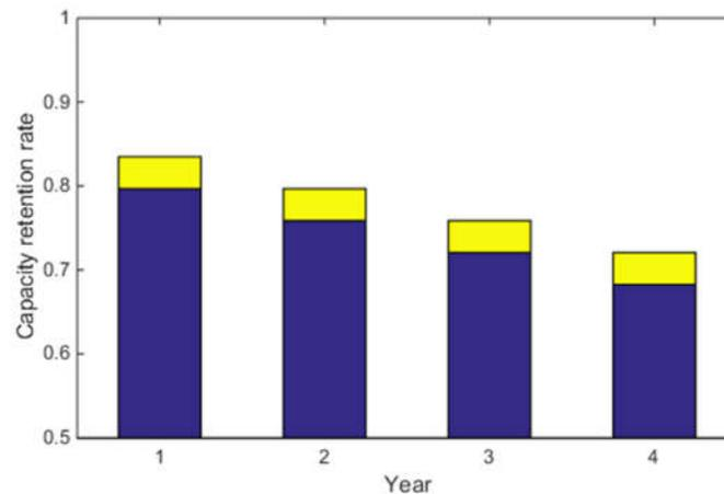
**Figure 7.** Storage battery capacity decays year by year.
