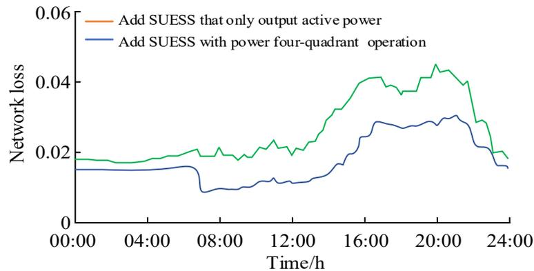
Figure 14. Two cases of the distribution network loss.
