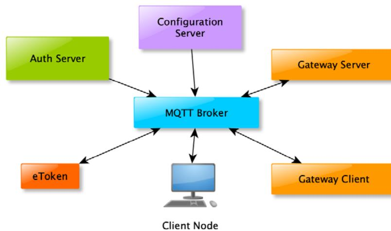
Figure 2. Message Queuing Telemetry Transport (MQTT) interconnects all the elements.
