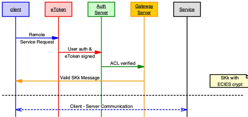
Figure 4. Message sequence chart (MSC) between the elements of the system.
