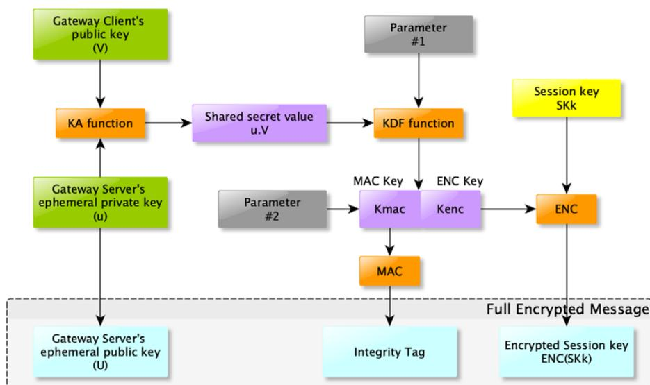
Figure 3. Scheme used to encrypt a session key.
