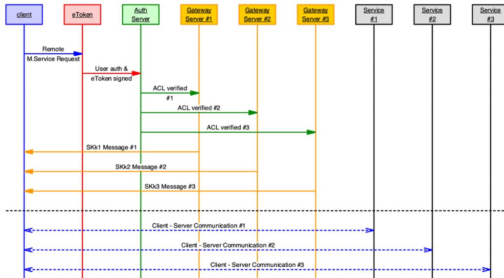
Figure 5. Message sequence chart between the elements of the system in a multiservice request.
