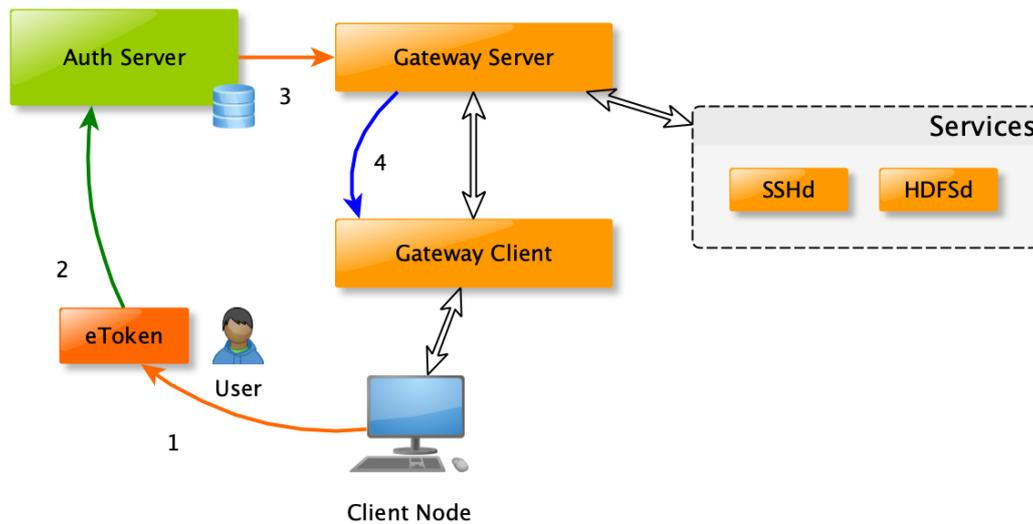
Figure 1. Main elements of the authentication and communication system.
