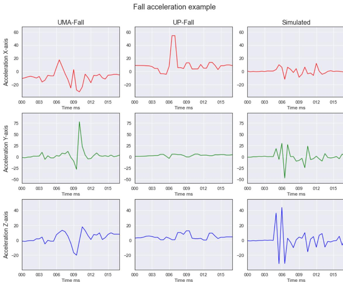
**Figure 5.** Unscaled accelerations for a forward fall event from the UMA-Fall dataset (**left**), UP-Fall dataset (**center**) and our simulated dataset (**right**), on the three axis.
