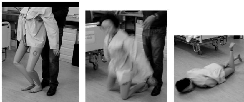
**Figure 1.** Syncope fall sequence using a dummy. From left to right: initial position, impact of the knees with the ground, and end position on the ground.
