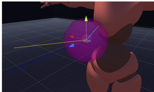
**Figure 4.** Forces decomposition in the simulator. In *blue*, original force; *cyan*: random point added to the original force; *yellow*: normalized addition of previous forces (final force applied).
