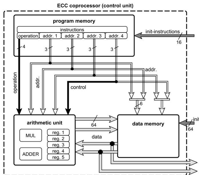
Figure 2. Block diagram of the ECC processor.
