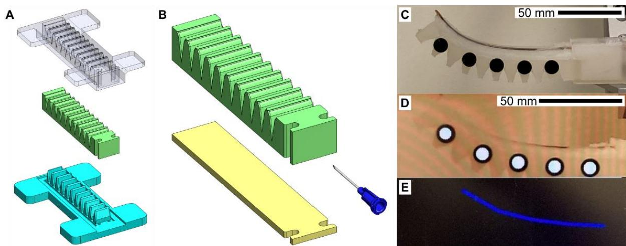
**Figure 1.** Soft finger actuator. (A) Actuator component (green) fabricated between stacked molds (blue, transparent). (B) Two actuator components before bonding. Green and yellow layers can be different material (different moduli) to prescribe actuator performance. Luer-lock needle (blue) inserted for pneumatic operation. (C) Actuator partially inflated instrumented with tracking markers. (D) Markers as tracked by software. (E) Finger position as interpreted by visual servoing system.
