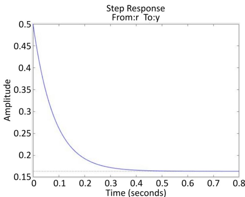
**Figure A2.** Step response of the system when  $K_p = 2$  and  $K_d = 0.5$ .
