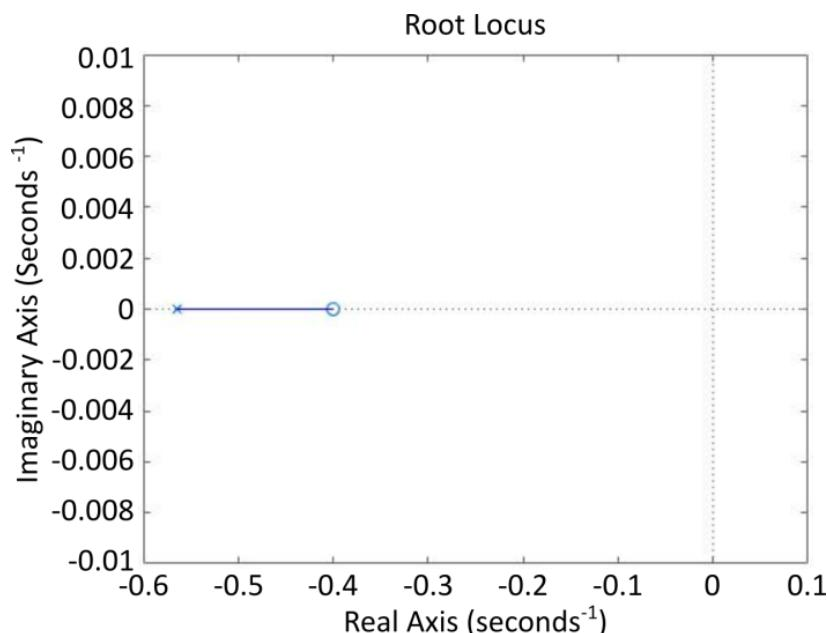
**Figure A1.** Root locus of the negative feedback loop system transfer function when  $K_p = 20$  and  $K_d = 50$ . The system has a singular pole and singular zero.
