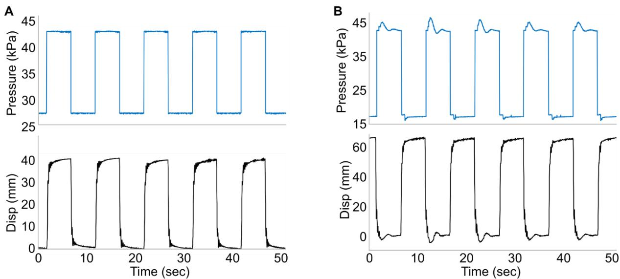
**Figure 4.** Square wave input, two approaches. (A). Pressure and displacement vs. time for approach 1 (Passive impedance). Pressure alternates between high and low setpoints as square wave. Infill and vent line impedances have been tuned to minimize ringing while maximize speed to setpoint. (B). Pressure/displacement curves for approach 2 (Visual servoing feedback control). The system is programmed to alternate the Y-height of the most distal marker between two setpoints.
