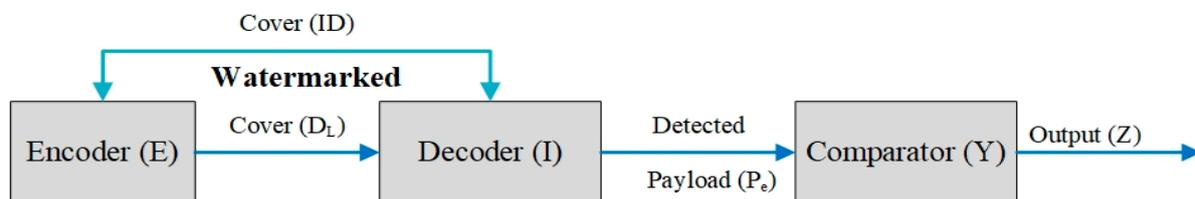
**Figure 1.** General watermarking system for multimedia objects [19].
