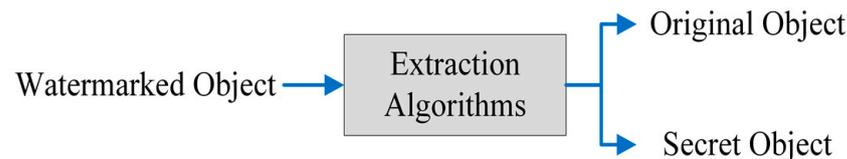
**Figure 5.** The watermark extraction procedure.
