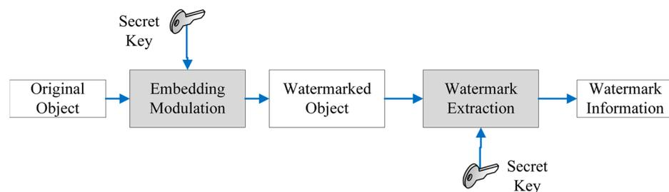
**Figure 2.** The watermarking Technique.
