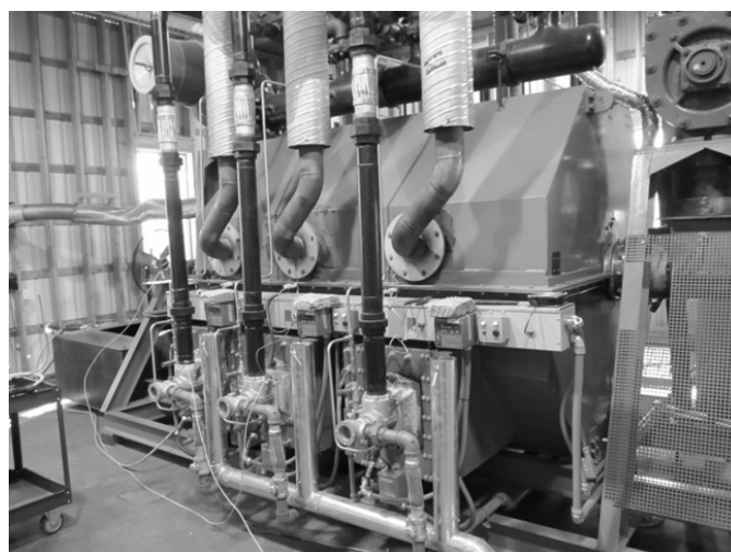
Figure 1. The Tucker Engineering Associates (TEA) gasifier used in this study. Photo: RMRS.
