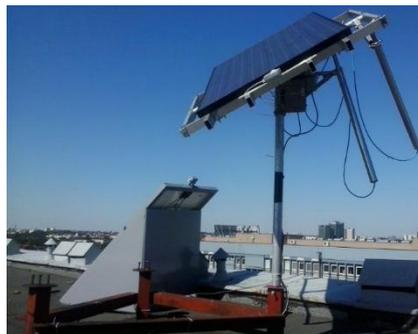
**Figure 1.** Two-axis tracking system with photovoltaic module, radiation power density meter and microinverter.
