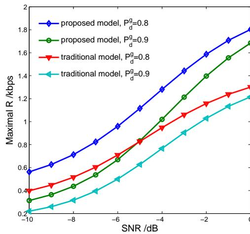
Figure 9. Maximal throughput versus spectrum sensing models.
