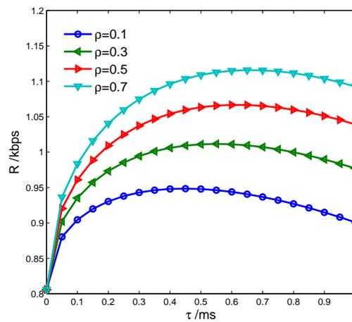
Figure 5. Throughput changed with sensing time.
