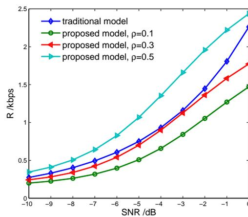
Figure 7. Throughput versus spectrum sensing models. SNR: signal to noise ratio.
