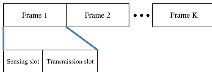
Figure 2. Traditional frame structure.
