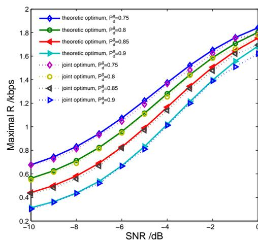
Figure 8. Maximal throughput versus theoretic optimum and joint optimum.
