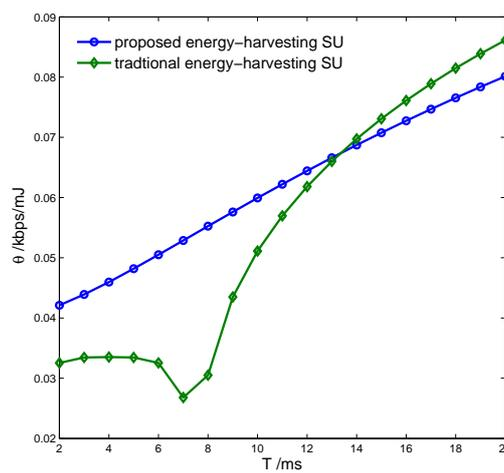
Figure 10. Energy-harvesting efficiency versus frame duration. SU: secondary user.
