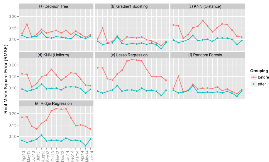
Figure 5. Average RMSE values of seven individual machine learning models' point forecasts before and after grouping of data by hours of the day. Results for: (a) decision tree; (b) gradient boosting; (c) KNN (distance); (d) KNN (uniform); (e) lasso regression; (f) random forests; and (g) ridge regression.
