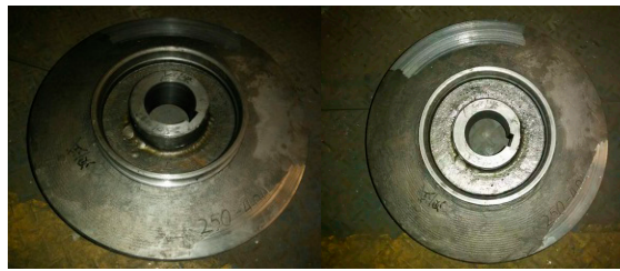
Figure 22. The casted impeller.
