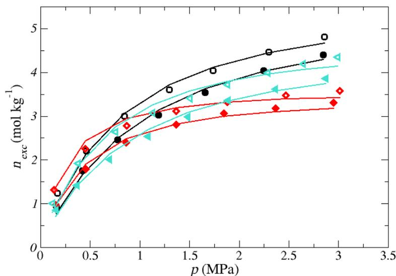
**Figure 2.**  $\text{CH}_4$  adsorption isotherms for the three olive stone-based activated carbons: AC- $\text{H}_3\text{PO}_4$  (black circles), AC- $\text{CO}_2$  (red diamonds) and AC- $\text{H}_2\text{O}$  (turquoise triangles). Open symbols represent the adsorption data at 303.15 K, while the data at 323.15 are shown by the filled symbols. Uncertainties:  $\Delta p = 0.01 \text{ MPa}$ ,  $\Delta T = 0.2 \text{ K}$ . The obtained Langmuir fitting isotherms are shown by the solid lines.
