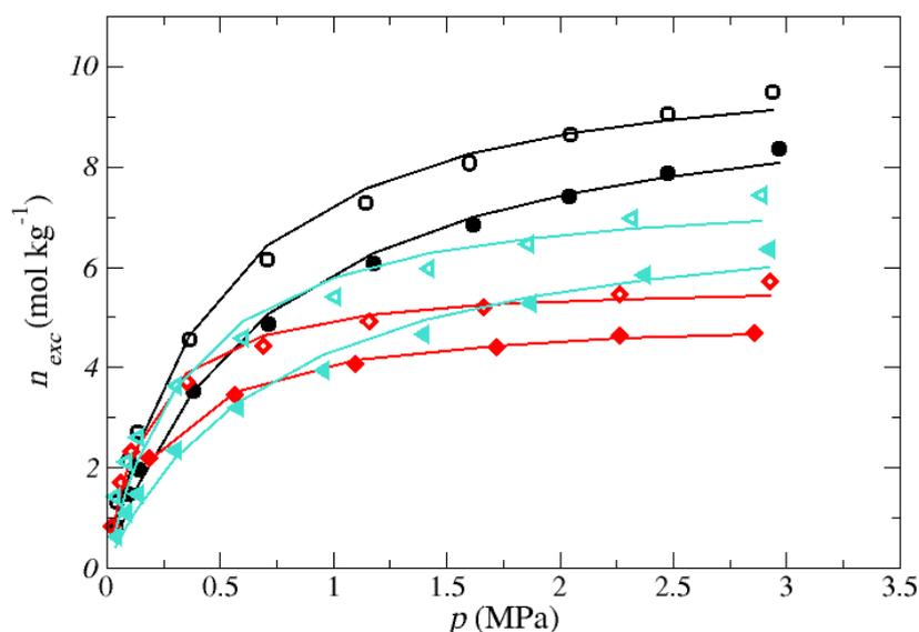
**Figure 3.** CO<sub>2</sub> adsorption isotherms for the three olive stone-based activated carbons: AC-H<sub>3</sub>PO<sub>4</sub> (black circles), AC-CO<sub>2</sub> (red diamonds) and AC-H<sub>2</sub>O (turquoise triangles). Open symbols represent the adsorption data at 303.15 K, while the data at 323.15 are shown by the filled symbols. Uncertainties:  $\Delta p = 0.01$  MPa,  $\Delta T = 0.2$  K. The obtained Langmuir fitting isotherms are shown by the solid lines.
