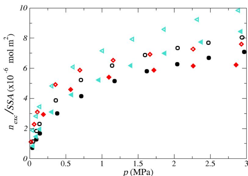
**Figure 4.** SSA normalized CO<sub>2</sub> adsorption isotherms of the activated carbons: AC-H<sub>3</sub>PO<sub>4</sub> (black circles), AC-CO<sub>2</sub> (red diamonds) and AC-H<sub>2</sub>O (turquoise triangles). Open symbols represent the adsorption data at 303.15 K, while the data at 323.15 are shown by the filled symbols 323.15 K.
