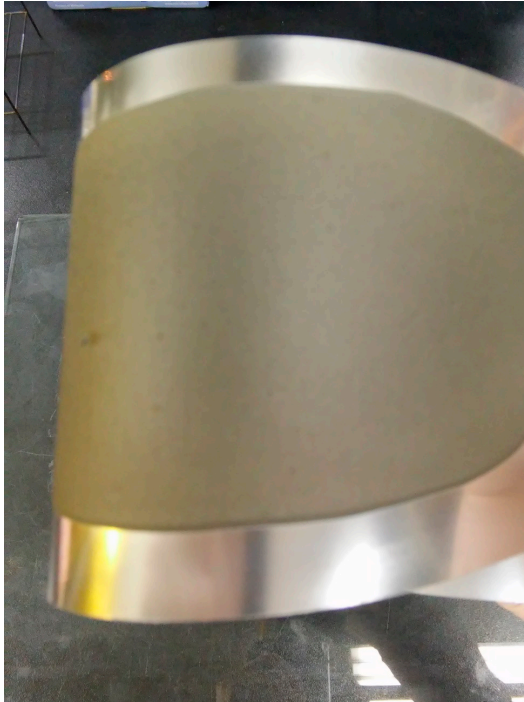
Figure S3. Bending test for cathode composite layer attached to the SUS plate and resulted in no cracks at 360° bending condition.
