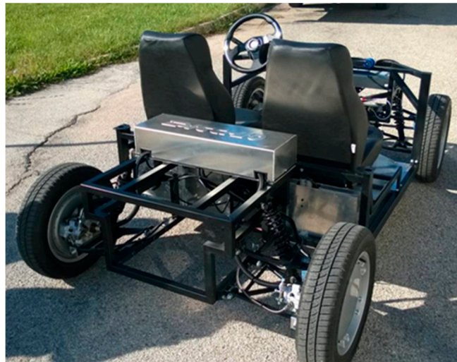
Figure 2. Electric motors are the powertrain of the Hi-Quad quadricycle, and they are placed inside the rear wheels. The inverters are inside the metal box behind the two seats, the battery pack is divided into two parts, and they are inside the aluminum packages that are located underneath the seats.
