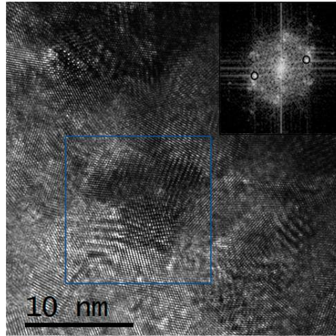
**Figure S2:** TEM micrograph of a Pt grain deposited on nickel by spontaneous galvanic displacement, after 1 min deposition. Moire fringes indicate the presence of two different crystalline patterns and the FFT in the inset shows the presence of spots (marked with black circles) corresponding to a plane distance of 2.2 Å, which is the value of (111) planes of Pt. The other spots are the pattern of NiO.
