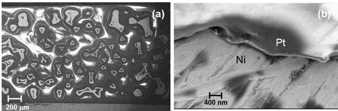
**Figure S1:** (a) Cross sectional SEM micrograph of the Ni foam after 8 min Pt deposition. (b) SEM image at higher resolution, showing the Pt layer on the Ni surface.
