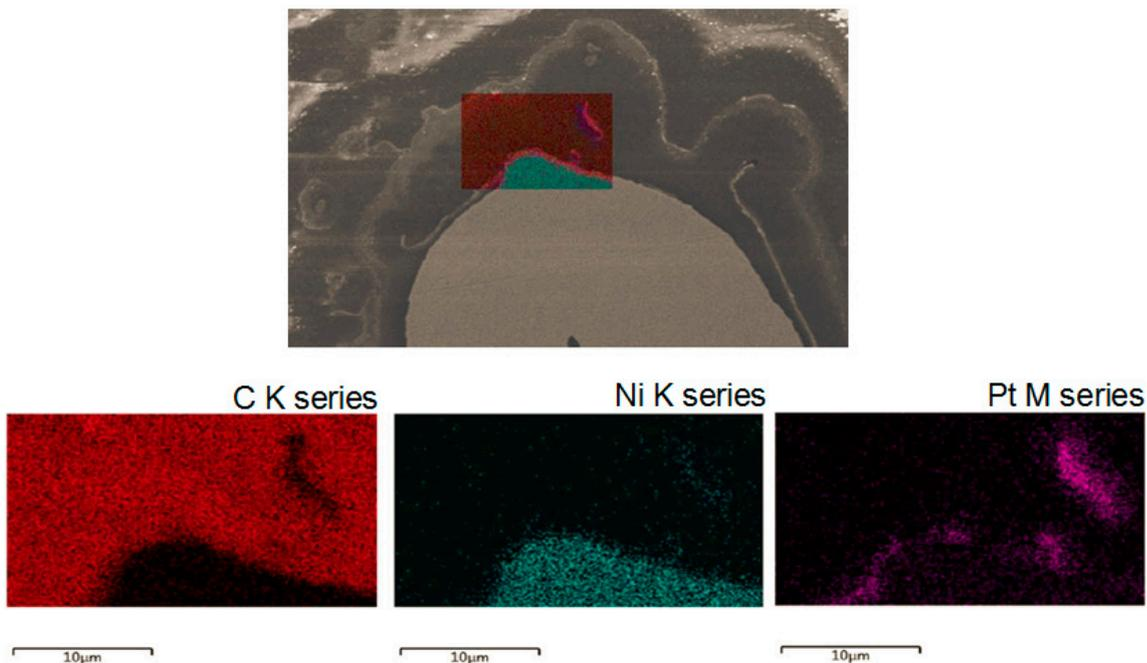
**Figure S3:** Cross section SEM image of a strut of Ni foam A after Pt deposition for 16 min. The elemental analysis shown in colour maps indicate the presence of a Pt film at the Ni surface, partially detached in some regions.
