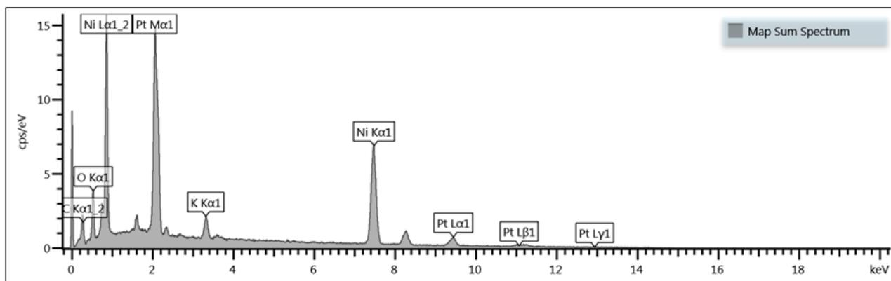
**Figure S4.** EDX spectrum acquired on the external surface of the Ni foam (sample A), after Pt deposition for 8 min.
