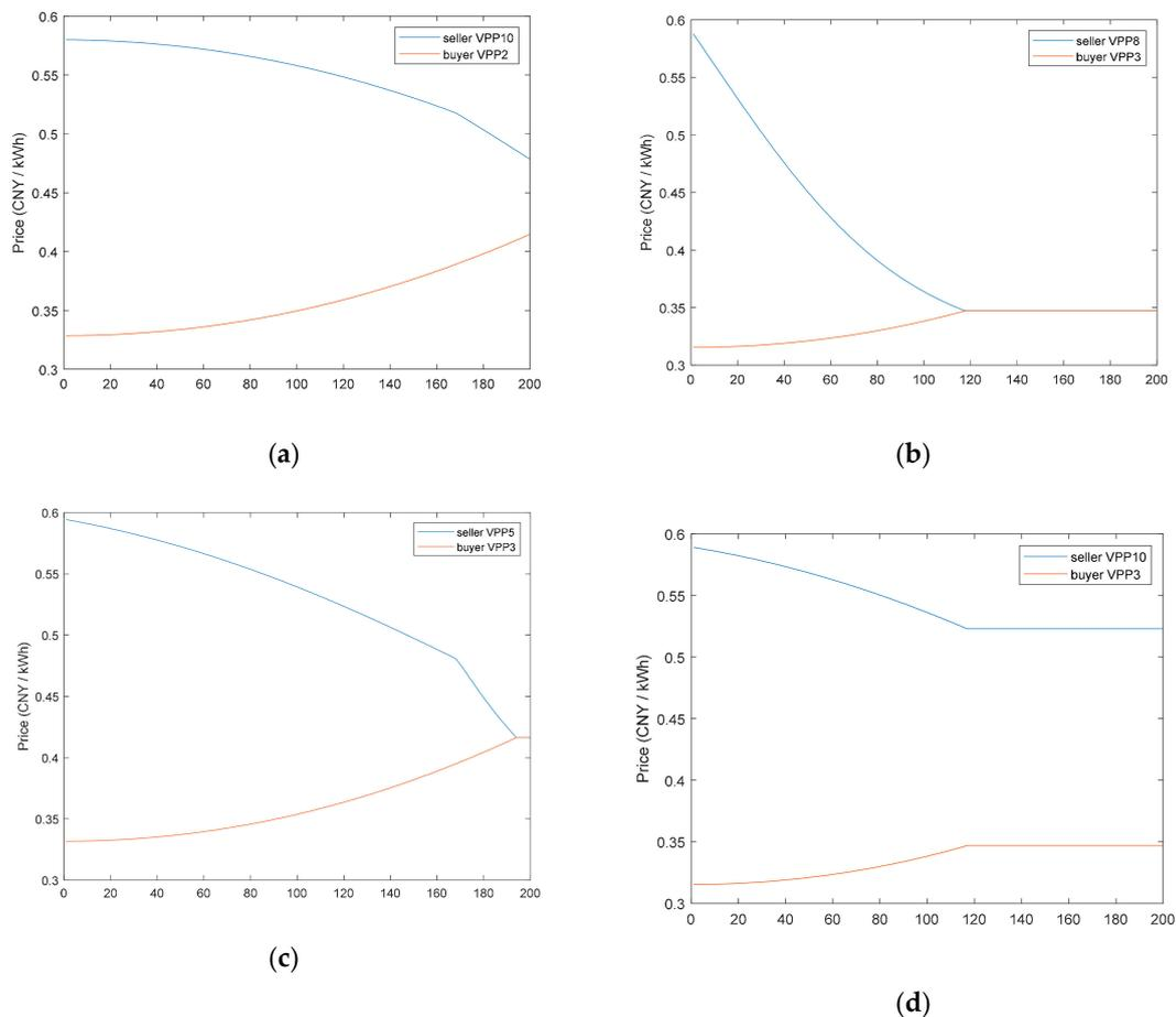
**Figure 7.** Price bidding process in the first round of P2P negotiation ( $R = 1$ ): (a) VPP<sub>2</sub> vs. VPP<sub>10</sub>,  $t = 1$ ; (b) VPP<sub>3</sub> vs. VPP<sub>8</sub>,  $t = 2$ ; (c) VPP<sub>3</sub> vs. VPP<sub>5</sub>,  $t = 1$ ; (d) VPP<sub>3</sub> vs. VPP<sub>10</sub>,  $t = 2$ .
