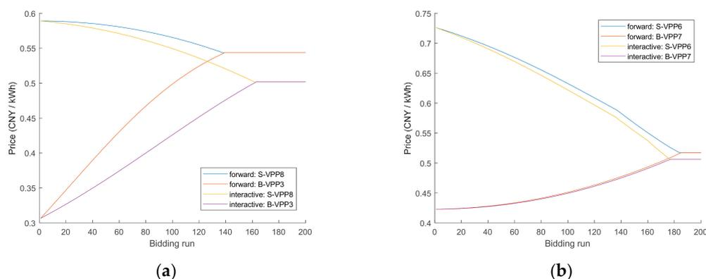
**Figure 10.** The price bidding process of P2P negotiation under two different mechanisms ( $R = 1$ ): (a) VPP<sub>8</sub> vs. VPP<sub>3</sub>,  $t = 1$ ; (b) VPP<sub>6</sub> vs. VPP<sub>7</sub>,  $t = 2$ . Figure 10 shows the price bidding processes of two typical buyer–seller pairs in the P2P negotiation.
