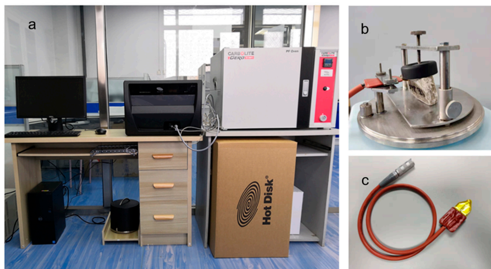
Figure 10. Schematic diagram of the thermal conductivity measurement principle: (a) Hot disk analyzer and the operating platform; (b) Testing of the rock samples according to the transient flat heat source method; (c) Thin-layer, disc-shaped probe.
