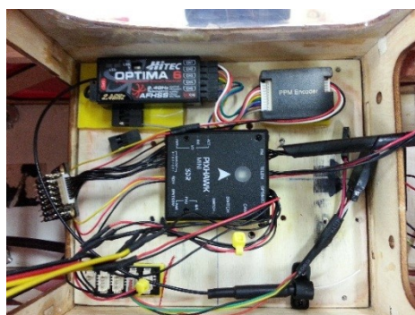
Figure 2. Control system and sensors used in the Kadet Senior UAV.
