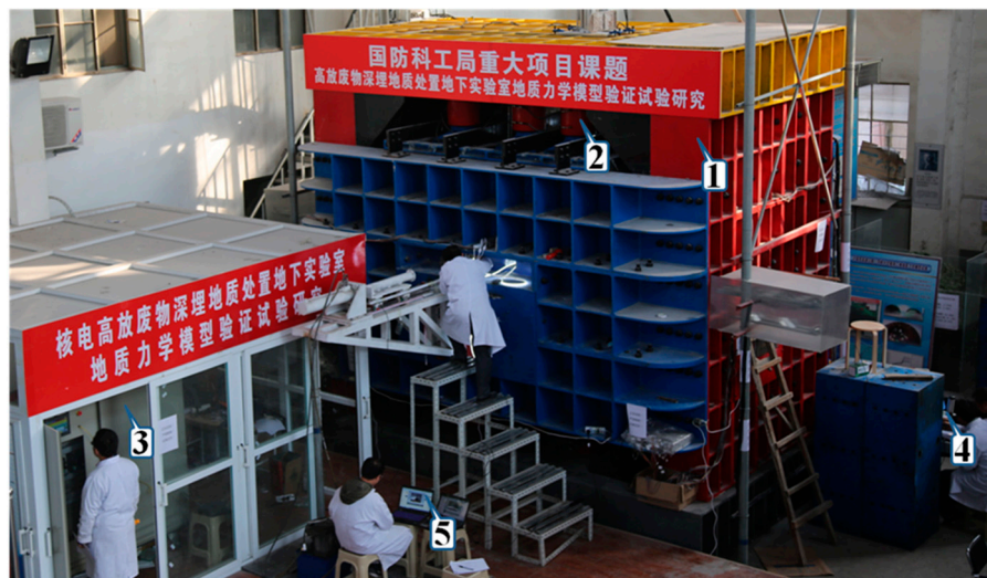
Figure 7. Picture of the model test system after assembly. 1: Combined bench counterforce device; 2: ultrahigh-pressure true 3D non-uniform loading/unloading device; 3: intelligent hydraulic loading/unloading control system; 4: automatic model displacement test system; and 5: high-definition multi-probe peeping system.
