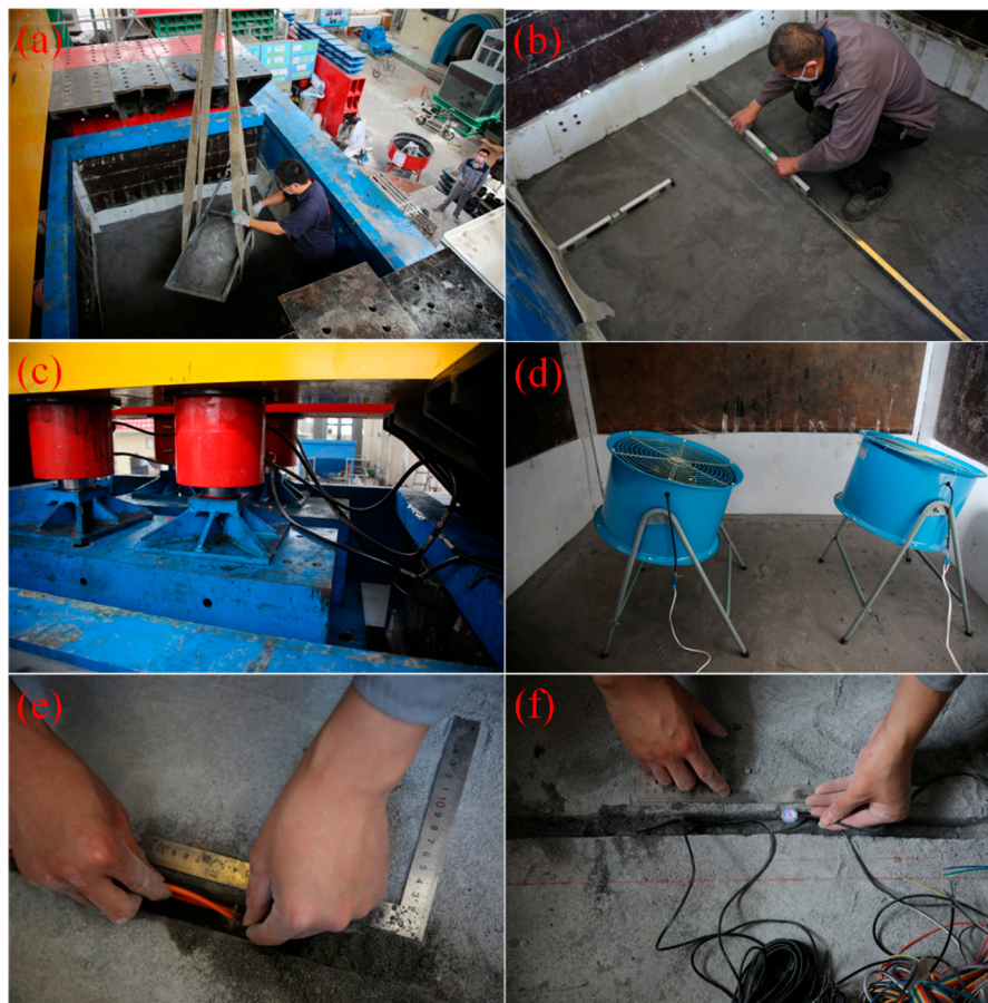
Figure 9. Photos of the construction of the physical model. (a) The mixed material is poured evenly into the test system; (b) the material is spread evenly; (c) the material is compacted by the loading system; (d) materials are air-dried with electric fans; (e) the optical displacement sensor is embedded; and (f) the strain sensors are embedded.
