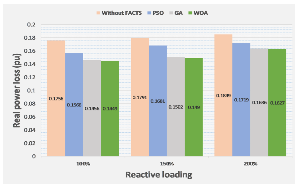
Figure 16. Comparison of real losses without and with FACTS in the IEEE-30 system using different techniques.
