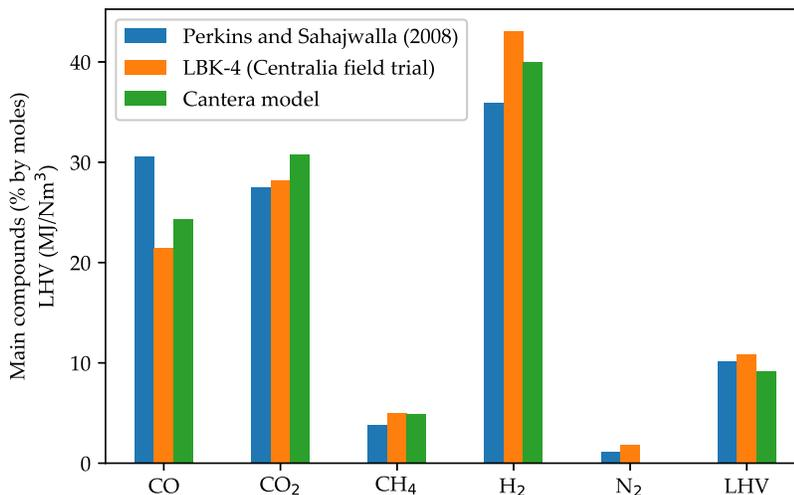
**Figure 5.** Comparison of our simulation results on the Centralia Large Block experiment LBK-4 ( $T = 630\text{ }^{\circ}\text{C}$ ,  $p = 0.125\text{ MPa}$ , stoichiometric ratio = 0.3) against field data [58] and the kinetic modeling results of Perkins and Sahajwalla [53].
