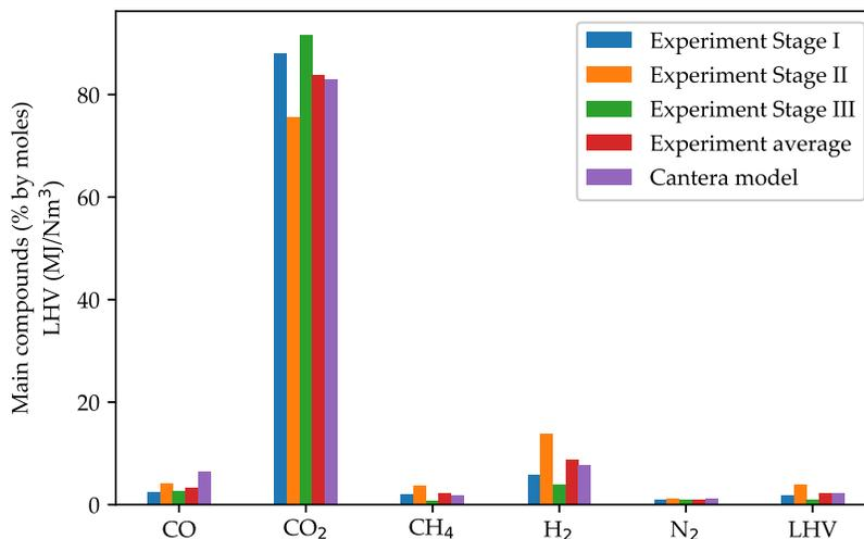
**Figure 4.** Comparison of average gas compositions for the three gasification stages and the average total gas composition of the Oltenia ortho-lignite experiment [52] against the results of our Cantera model ( $T = 580$  °C,  $p = 1$  MPa, stoichiometric ratio = 0.35).
