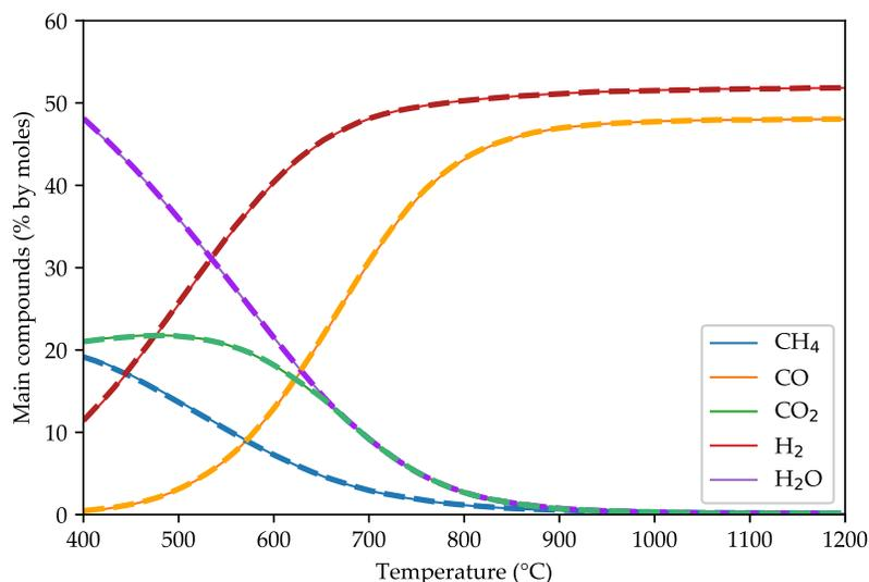
**Figure 2.** Simulation results for the synthesis gas equilibrium composition plotted as function of process temperature for the pine sawdust pyrolysis test at 0.1 MPa (dashed lines) compared to literature data [16] (solid lines).
