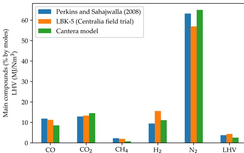
**Figure 6.** Comparison of our simulation results on the Centralia Large Block experiment LBK-5 ( $T = 585\text{ }^{\circ}\text{C}$ ,  $p = 0.125\text{ MPa}$ , stoichiometric ratio = 0.3) against field data [58] and the kinetic modeling results of Perkins and Sahajwalla [53].
