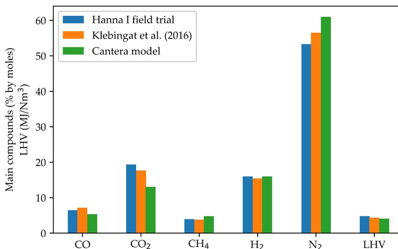
**Figure 7.** Comparison of our simulation results ( $T = 600$  °C,  $p = 0.48$  MPa, stoichiometric ratio = 0.12) against the Hanna I experiment field data [60] and the thermodynamic modeling results of Klebingat et al. [37].
