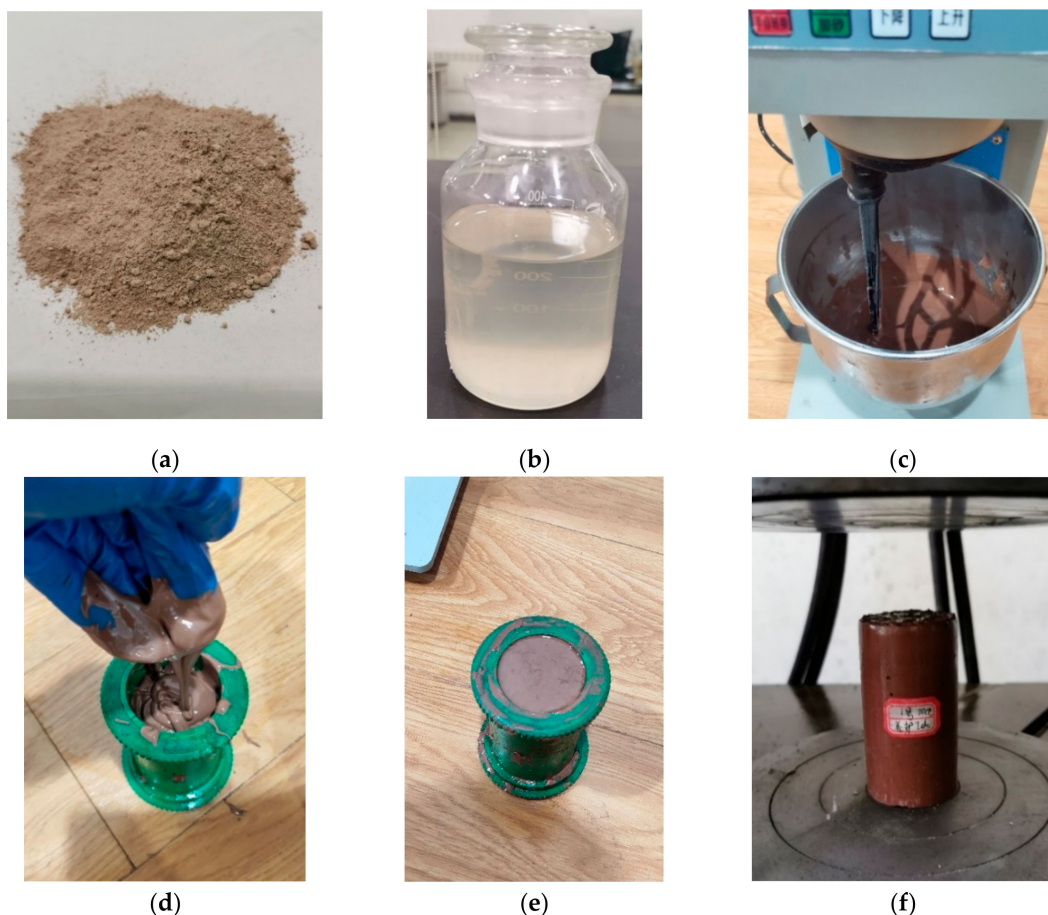
Figure 2. Preparation process of coal gangue-based geopolymer (CGGP) specimen: (a) 700 °C-CG; (b) Alkali medium; (c) Mixing and stirring; (d) Filling into mold; (e) Solidifying at room temperature; (f) Cured 700 °C-CGGP specimen.
