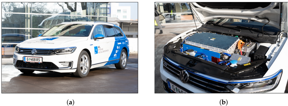
Figure 1. (a) The KEYTECH4EV fuel cell demonstrator vehicle, based on a VW Passat hybrid. (b) Engine bay with the retro-fitted fuel cell system.
