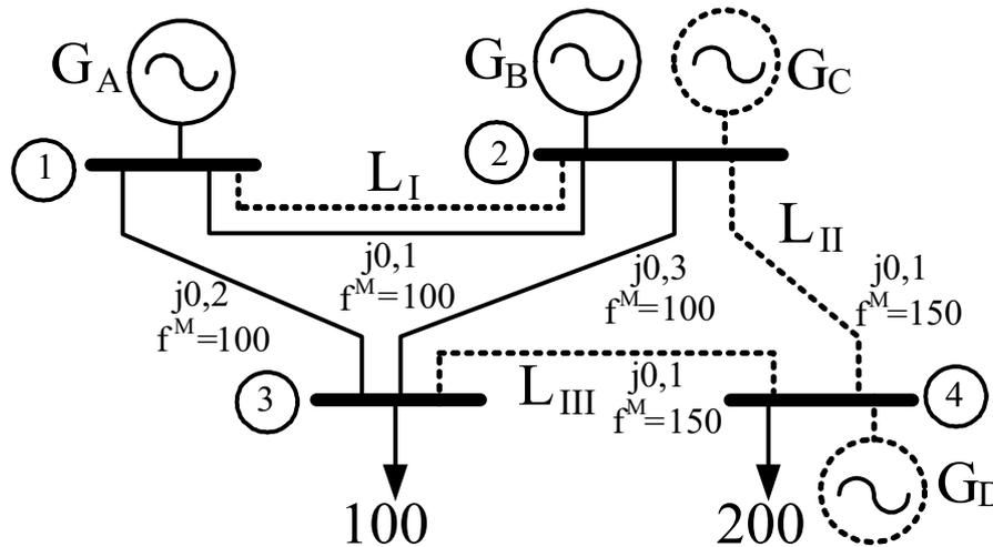
Figure 1. Power system example.
