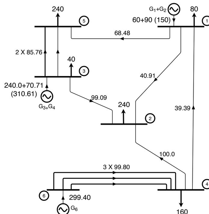
**Figure 4.** Power flow solution for the Garver power system.
