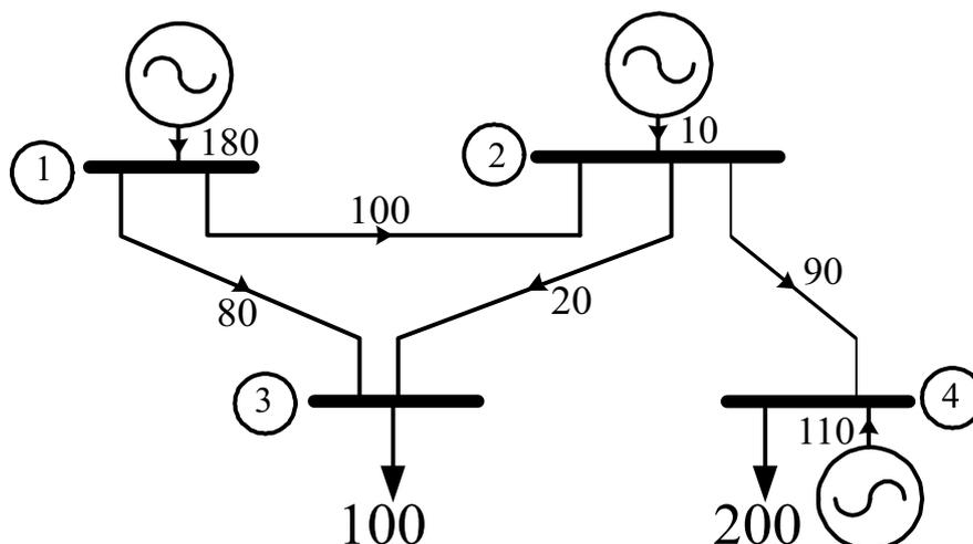
Figure 2. Power flow solution.
