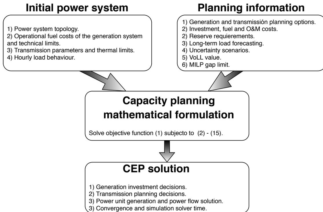
**Figure 3.** Capacity expansion planning framework.
