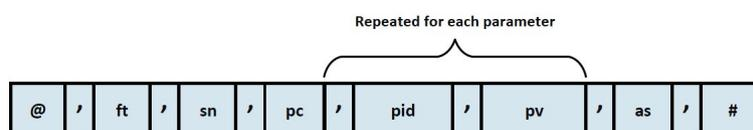
Figure 14. Data frame structure.
