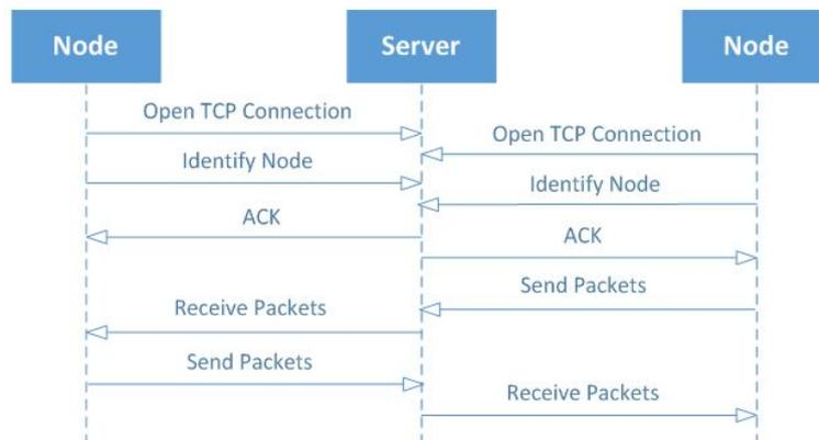
Figure 10. Sequence diagram for node to node communication.
