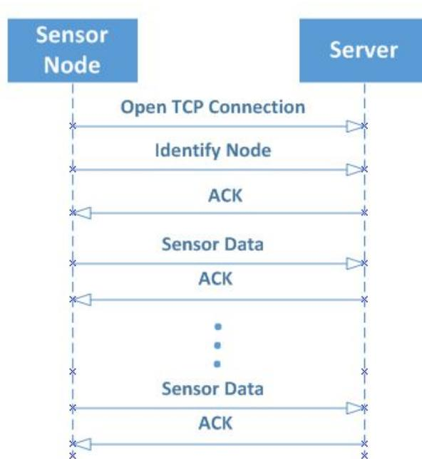
**Figure 6.** Sequence diagram for a sensor node. ACK: acknowledgement message.
