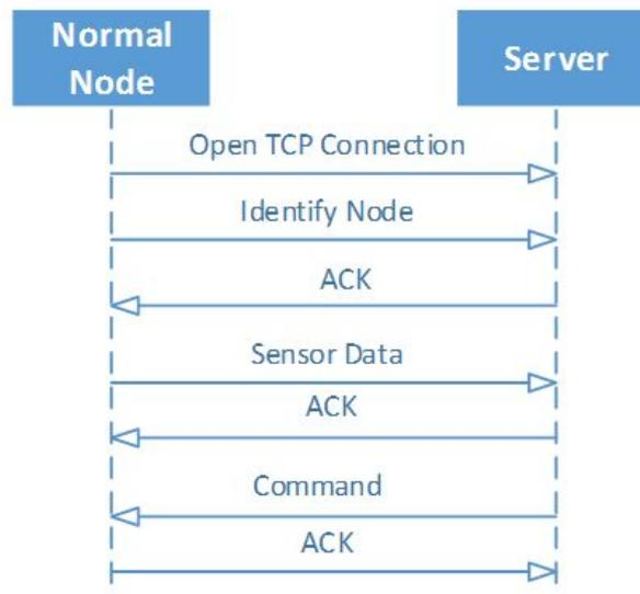
**Figure 8.** Sequence diagram of a normal node.
