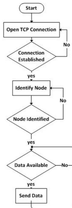
Figure 19. Sensor node flowchart.
