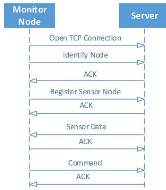
**Figure 9.** Sequence diagram of a monitor node.
