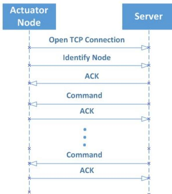
**Figure 7.** Sequence diagram for an actuator node.
