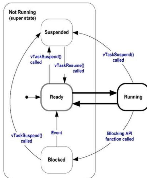
Figure 17. Task state diagram.
