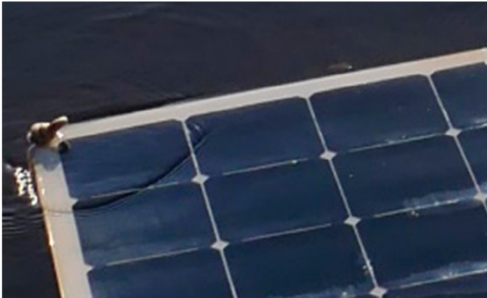
Figure 2. Closeup of floating photovoltaic/floatovoltaic (FPV) corner after deployment, showing water coverage from a modest wave (top left).
