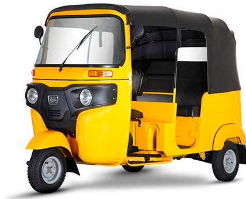
Figure 1. BAJAJ RE 205 cc motorized three-wheeler [3].
