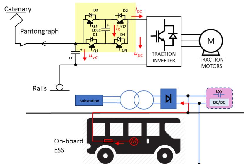
**Figure 7.** Topology of onboard-wayside supercapacitor hybrid energy storage system extracted adapted from [32].
