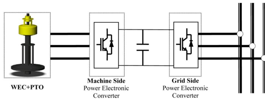
**Figure 16.** Simplified electrical diagram of a WEC+PTO with linear generator connected to the grid.
