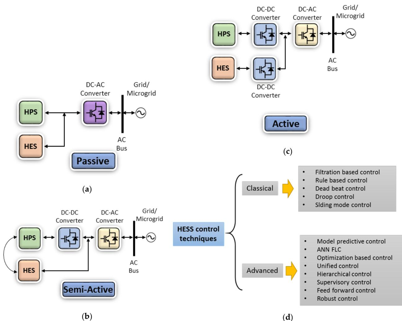
**Figure 17.** Main interconnection topologies for a HESS, formed by a high power storage (HPS) and a high energy storage (HES): (a) passive, (b) semi-active and (c) active adapted from [71]; (d) Classification of HESS control techniques adapted from [71].
